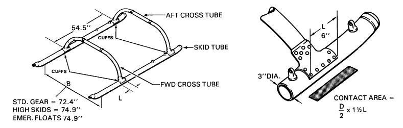
LANDING GEAR LOADING @ MAXIMUM GROSS WEIGHT – 3200 (POUNDS) BASED ON ONE "G" STATIC CONDITIONS AT AFT MOST STRUCTURAL CG LIMIT
