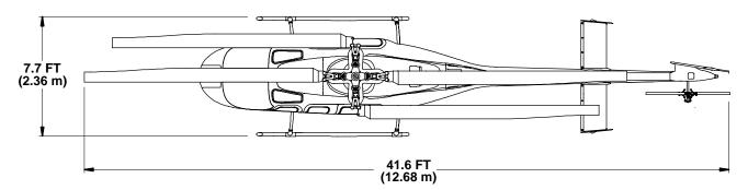
MINIMUM HANGAR SIZE\* ROTOR NOT FOLDED 25.1 FT X 36.6 FT [ 7.7 M X 11.2 M ]
