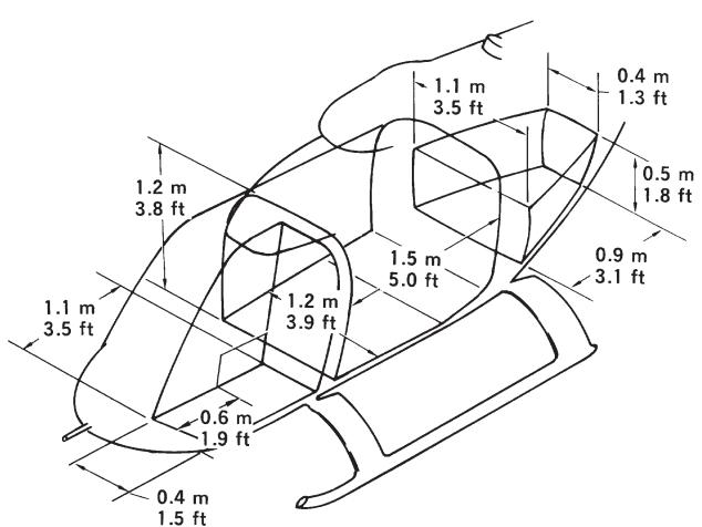
Approximate cargo space: Aft Cabin-2.4 cubic meters (85 cubic feet) Left front-0.6 cubic meters (20 cubic feet) Baggage compartment-0.45 cubic meters (16 cubic feet)
