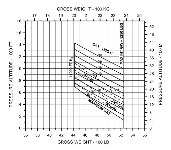
**NOTE:** TAKEOFF AND LANDING WITH OPTIONAL 5250 LB/2381 KG INTERNAL GROSS WEIGHT HAS NOT BEEN DEMONSTRATED AND IS NOT APPROVED ABOVE <u>11,000 FEET/3353 METERS</u> **DENSITY ALTITUDE**.
