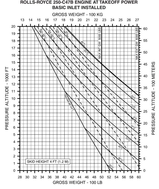
**NOTE:** TAKEOFF AND LANDING HAS NOT BEEN DEMONSTRATED AND IS NOT APPROVED ABOVE <u>17,000 FEET / 5182 METERS</u> **DENSITY ALTITUDE**.
