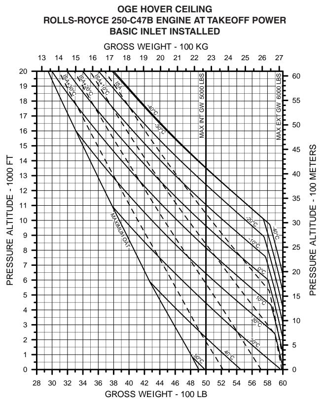
**NOTE:** TAKEOFF AND LANDING HAS NOT BEEN DEMONSTRATED AND IS NOT APPROVED ABOVE <u>17,000 FEET / 5182 METERS</u> **DENSITY ALTITUDE**.
