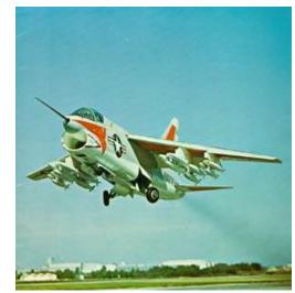
allow it to stay in the air for over 12 hours! The normal weapon load was around 15,000 pounds, which was carried on eight store stations, but the A-7A demonstrated the capability to carry 20,000 pounds of ordnance. An incredible mix of weapons and fuel loading produced varying radius-of-action capabilities within its 42,000-pound gross weight limit.
