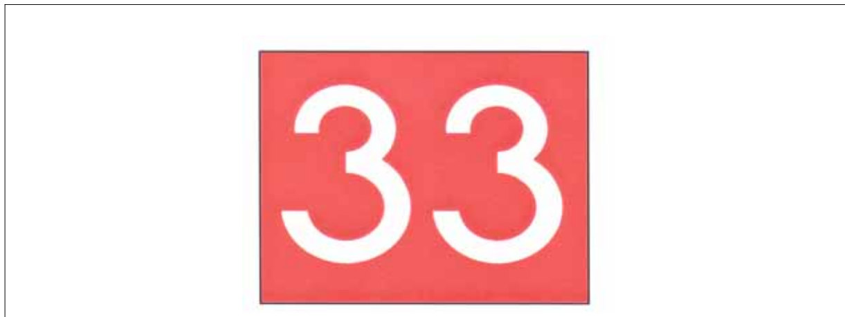
FIG AD 1.1-34 Holding Position Sign at Beginning of Takeoff Runway
