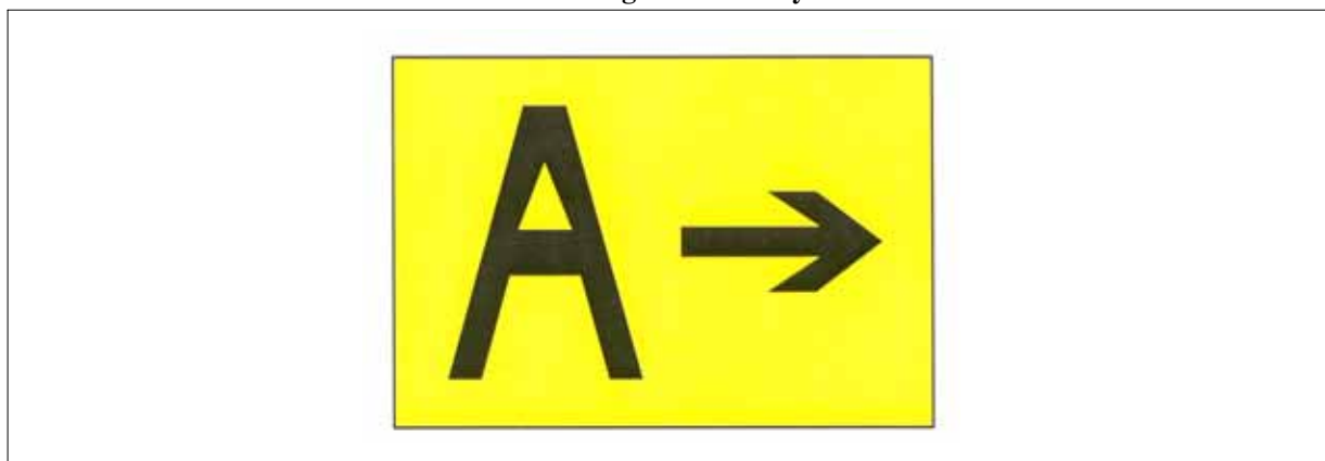
FIG AD 1.1-45 Direction Sign for Runway Exit
