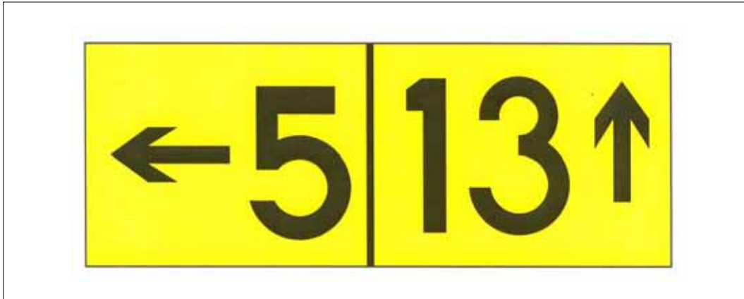
FIG AD 1.1-49 Destination Sign for Different Taxiing Routes to Two Runways
