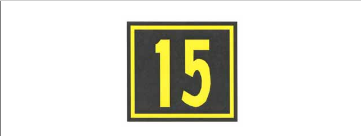
FIG AD 1.1-41 Runway Location Sign
