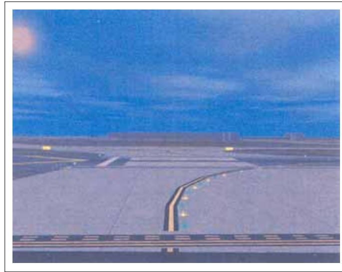
FIG AD 1.1-9 Taxiway Lead-On Light Configuration
