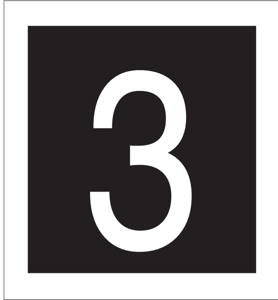
FIG AD 1.1-50 Runway Distance Remaining Sign Indicating 3,000 feet of Runway Remaining
