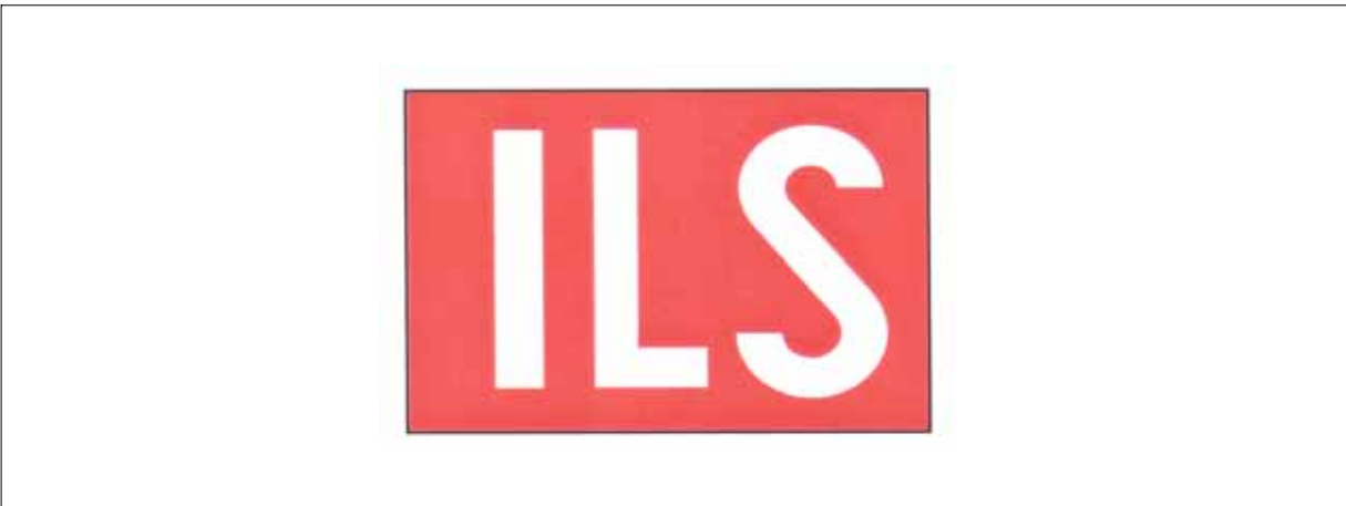
FIG AD 1.1-37 Holding Position Sign for ILS Critical Area
