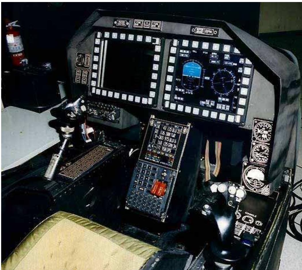
A new glass cockpit has been developed for the Super Cobra
