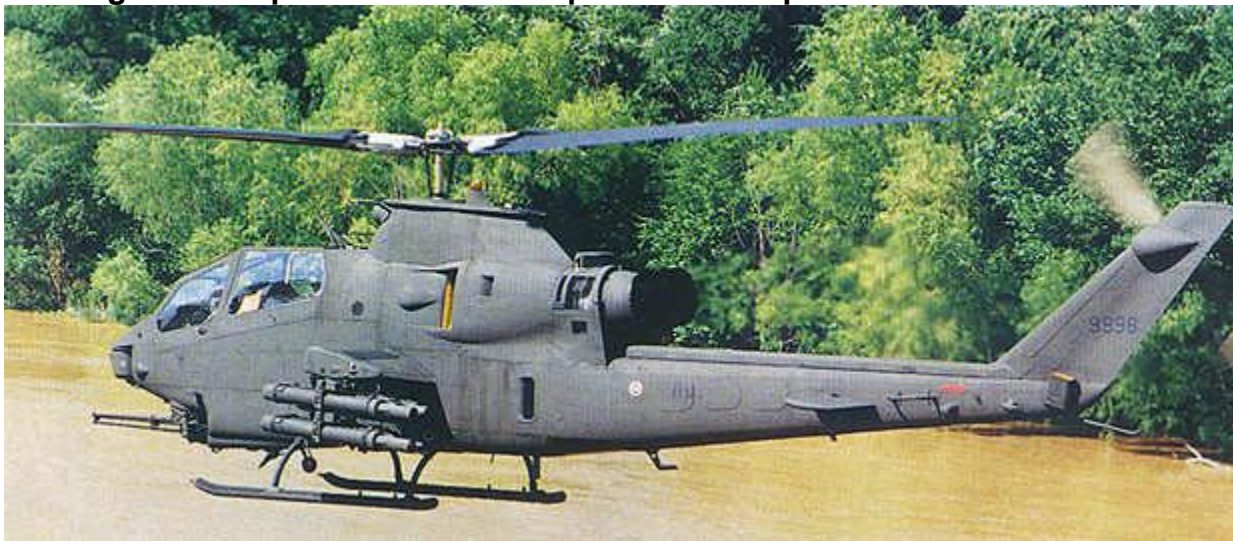
A Super Cobra AH-1F armed with TOW missiles.
