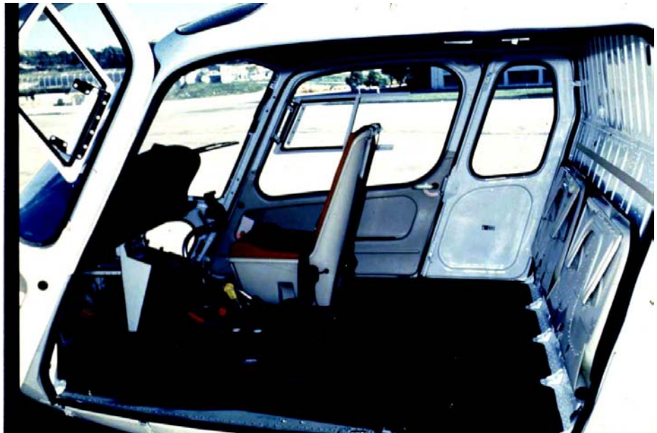
Internal cargo load transport lay-out
