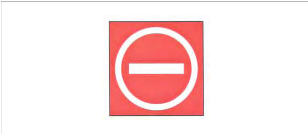
FIG 2-3-29 Sign Prohibiting Aircraft Entry into an Area
