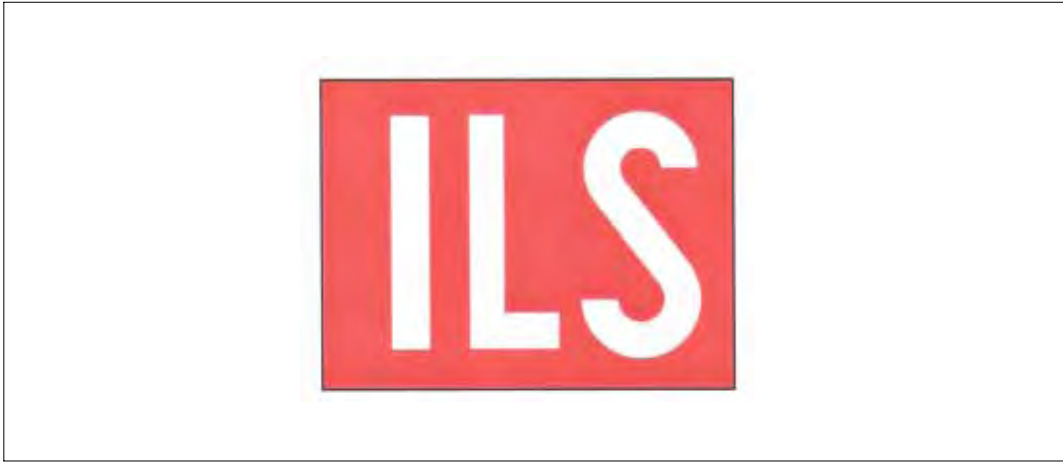
FIG 2-3-28 Holding Position Sign for ILS Critical Area
