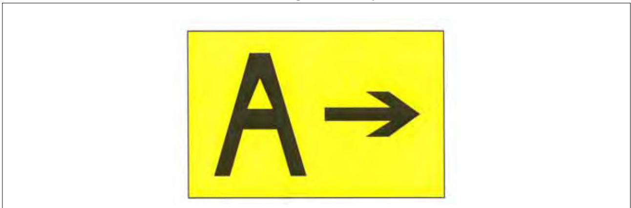
FIG 2-3-36 Direction Sign for Runway Exit
