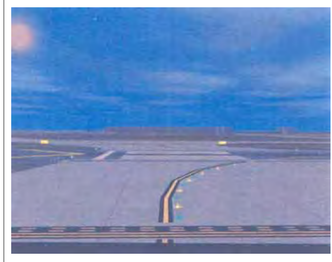
FIG 2-1-9 Taxiway Lead-On Light Configuration
