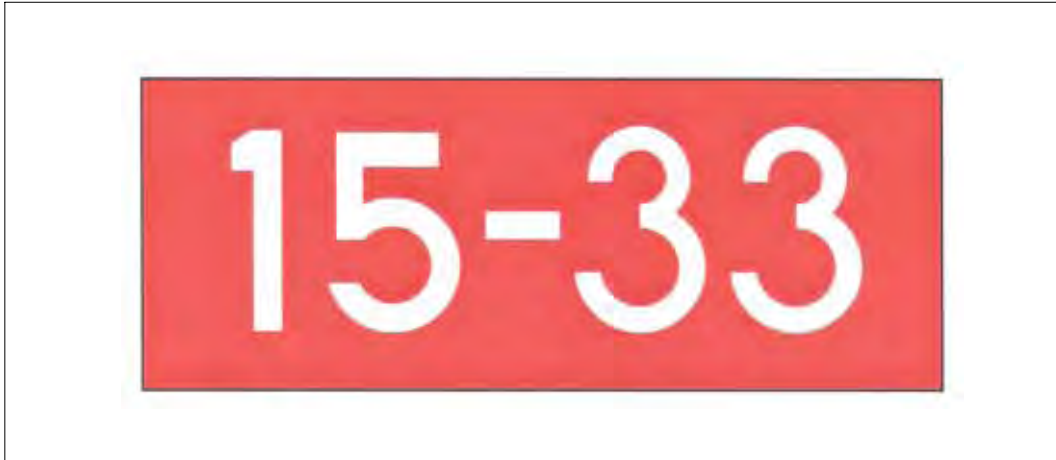
FIG 2-3-24 Runway Holding Position Sign
