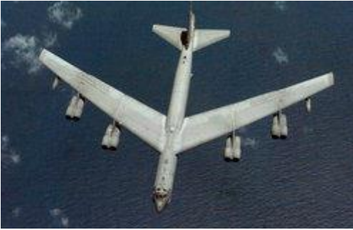
The high aspect ratio wing of a USAF B52 bomber
