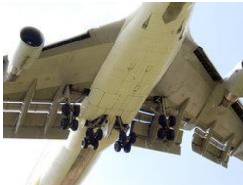
Wing and fuselage undercarriages on a Boeing 747 , shortly before landing
