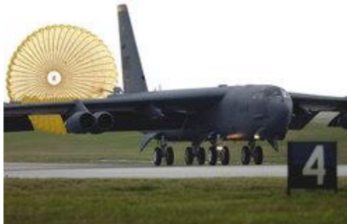
The dual tandem landing gear of a B-52 Stratofortress
