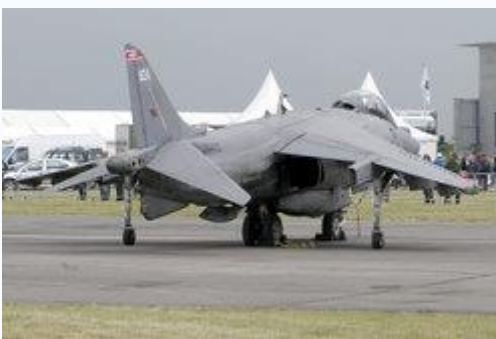
Hawker Harrier GR7 (ZG472) showing the two mainwheels in line astern under the fuselage and the smaller wheel near the tip of each wing.
