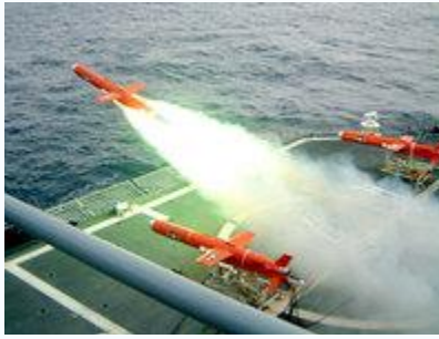
BMQ-74E Chukar target drone using JATO
