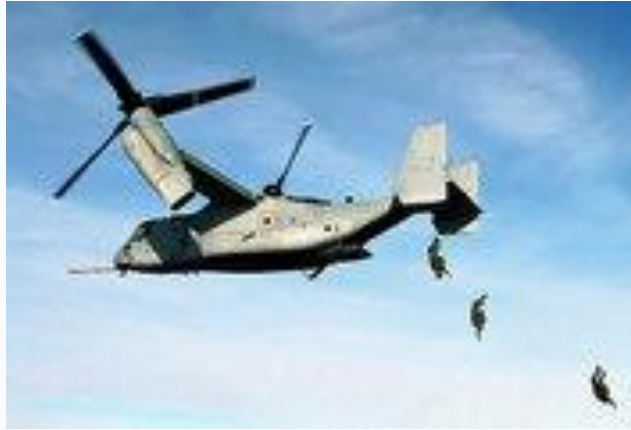
The Bell-Boeing V-22, an example of a tiltrotor aircraft
