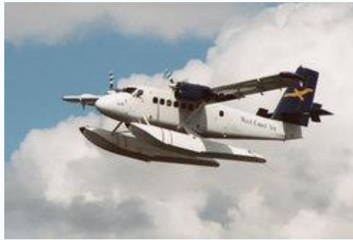
A turboprop -engine DeHavilland Twin Otter adapted as a floatplane
