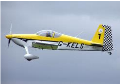
The Vans RV-7 fuselage is slender for high speed flight
