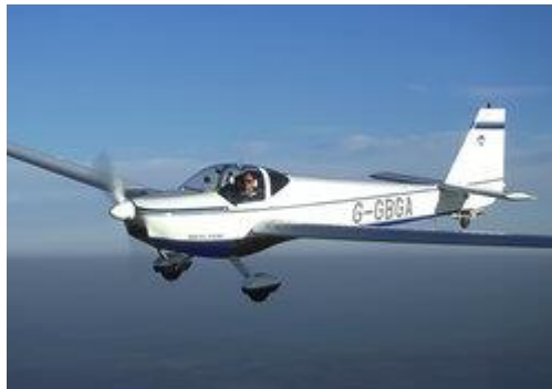
Scheibe SF25C - a typical old-style touring motorglider
