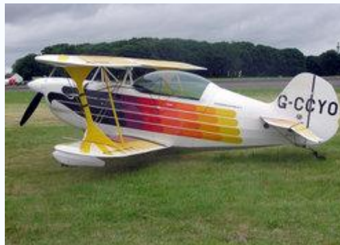
The fuselage can be short, and seemingly unaerodynamic, as in this Christen Eagle 2
