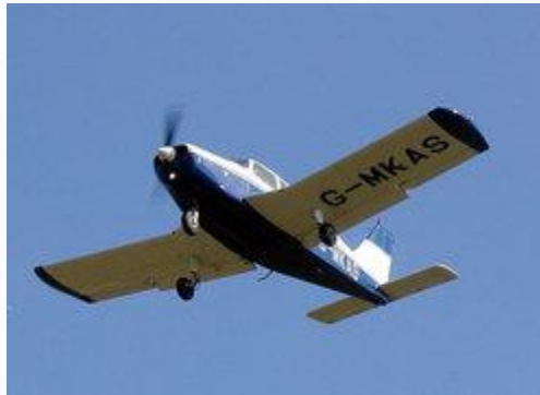
The low aspect ratio wing of a Piper PA-28 Cherokee
