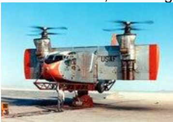
Ground testing the X-18 tiltwing
