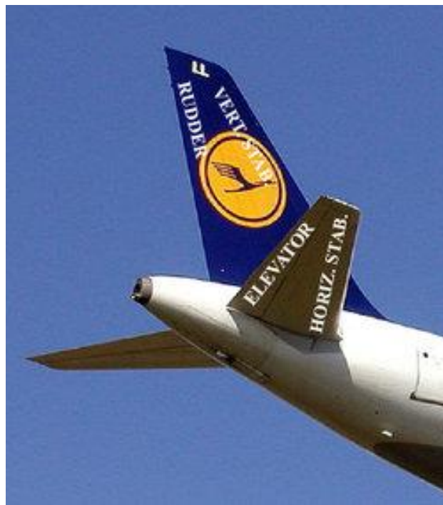
The tail of a Lufthansa Airbus A319, showing flight controls (Stab. means Stabiliser)
