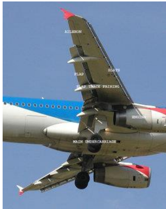
BMI Airbus A320, showing position of aileron, flap and slat flight controls . Click on the picture to read the labels more clearly
