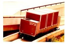
up to at least 3 mph. A draw bar and umbilical allows two-car trains to be operated.
