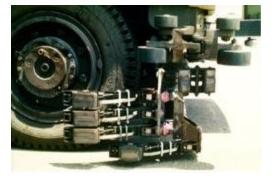
become entrapped under the switch rail, thus steering the vehicle through the switch. In a switch area, one wheel is always entrapped under a rail, providing protection against splitting a switch.
