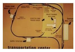
center there is a departure test track, used to ensure that vehicle safety features are functioning, and a ready track for vehicles awaiting dispatch into service. For layout, see the Transportation Center illustration.
