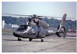
The Panther 800 was offered to the Army as a light utility helicopter. It is a variant of the Aerospatiale AS-565 and a sister ship to the Coast Guard HH-65. The Panther 800 had two Army T800 engines and an improved, state-of-the art cockpit.
