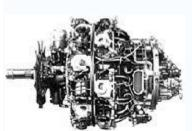
BMW 801 side view. Note the fan on the front (left) and large accessories section at the rear, which includes the supercharger.
