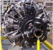
BMW 801 front view. Note the cooling fan (black). The three cylinders at the front are the propeller pitch drive, not part of the engine itself.
