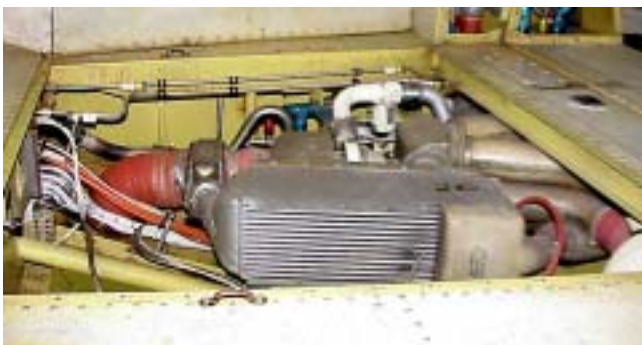
ECU EQUIPMENT [UNDER BAGGAGE COMPARTMENT FLOOR]
