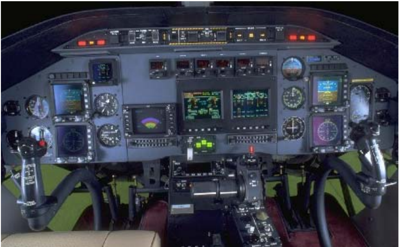
INTEGRATED INSTRUMENT DISPLAY SYSTEM (IIDS) - SHOWN WITH OPTIONAL EQUIPMENT
