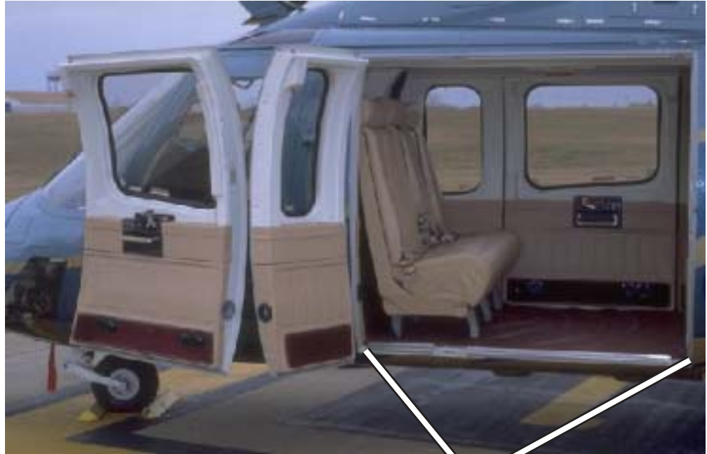
LITTER DOOR 54 INCHES [1.37 METERS] WIDE ACCESS
