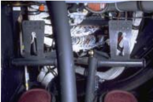
TOE BRAKES ↑ / ↓ PITOT-STATIC SWITCHES
