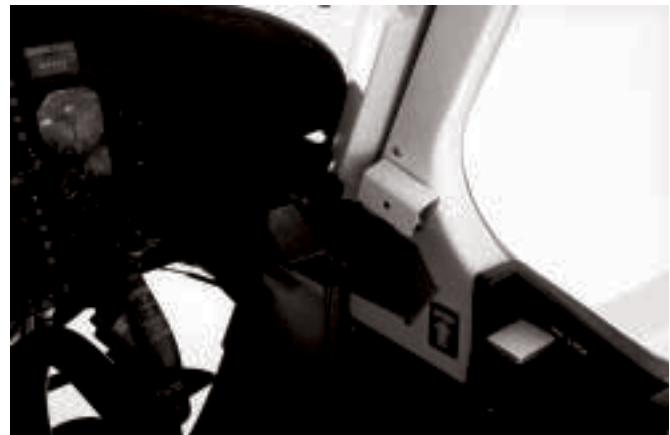
APPROACH PLATE HOLDER SWINGS AWAY IF NOT NEEDED
