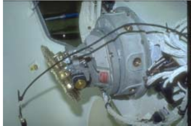
NOSE FRAHM SERVES AS MOUNT FOR OPTIONAL RADAR ANTENNA
