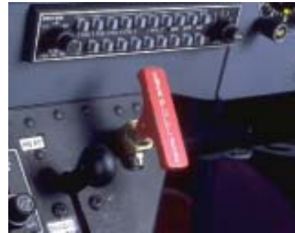
EMER. GEAR RELEASE ↑ / ↓ PARKING BRAKE
