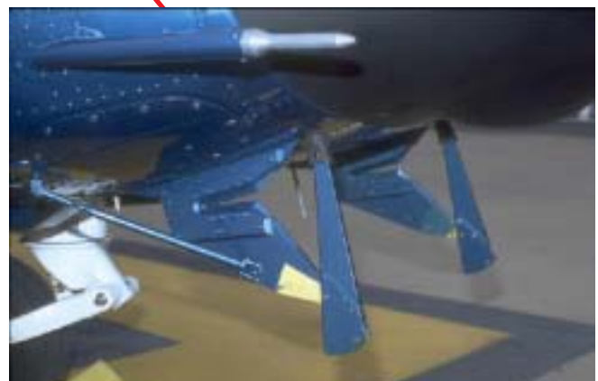
LOWER CUTTERS FOLD UP FOR GROUND HANDLING
