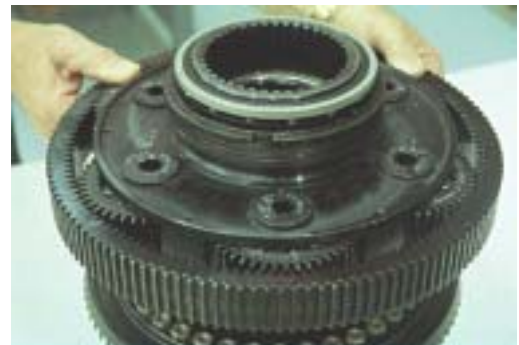
PLANETARY & RING GEAR SET
