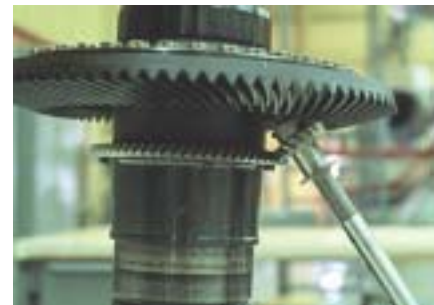
MAIN SPIRAL BEVEL COLLECTOR GEAR
