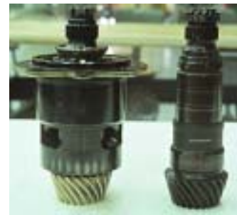
MAIN SPIRAL BEVEL COLLECTOR GEAR
