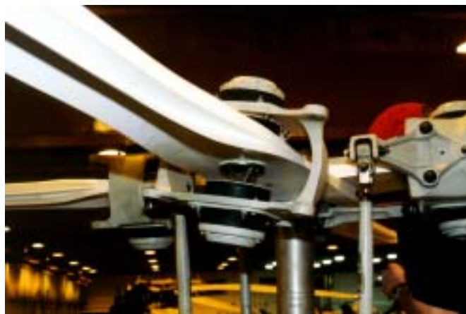
STACKED YOKES - PITCH CHANGE ADAPTER & PITCH HORN
