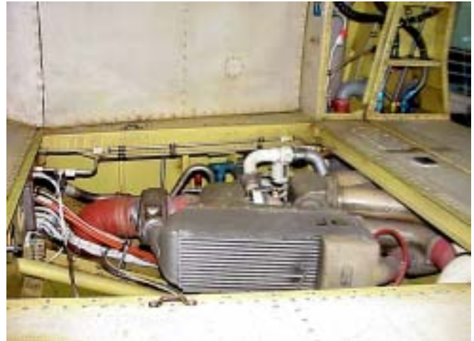
LOWER EQUIPMENT COMPARTMENT W/ OPTIONAL ENVIRONMENTAL CONT. UNIT
