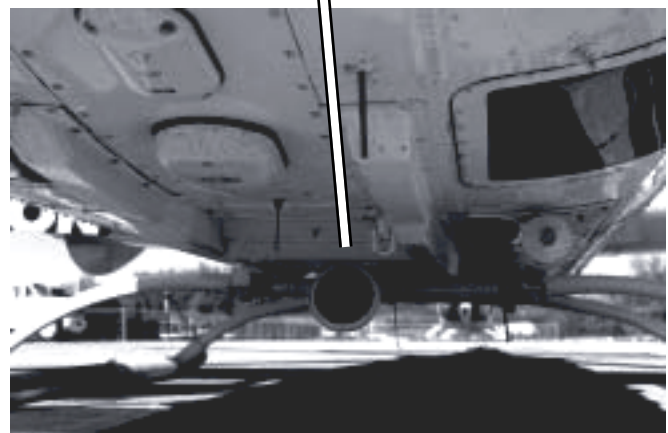
DIRECTIONALLY CONTROLLABLE LANDING/SEARCH LIGHT
