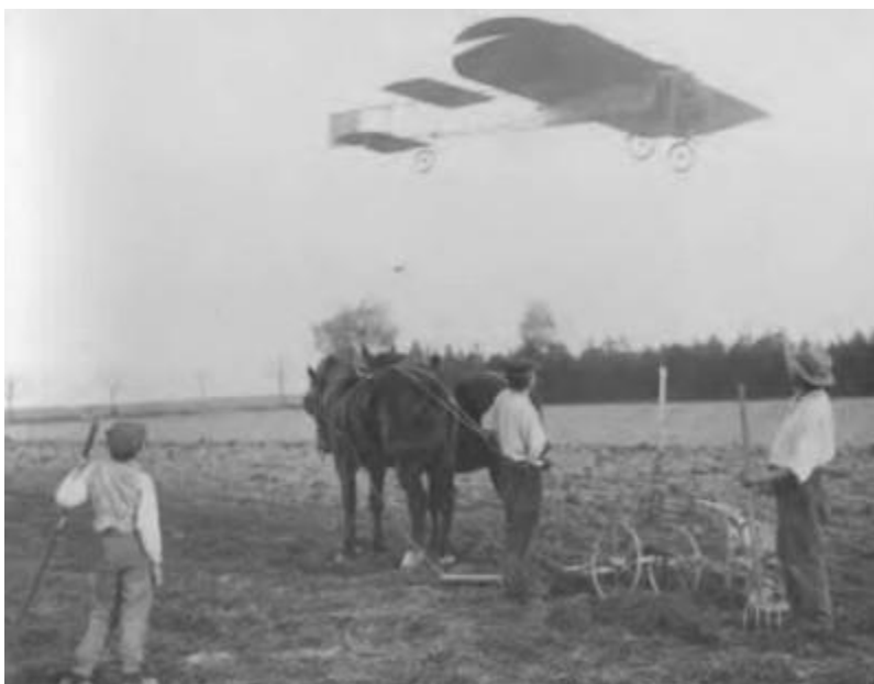
The Blériot VIII-bis near Dambron during 31 Oct 1908 cross country flight from Toury to Artenay. The wing-tip ailerons are clearly visible.
