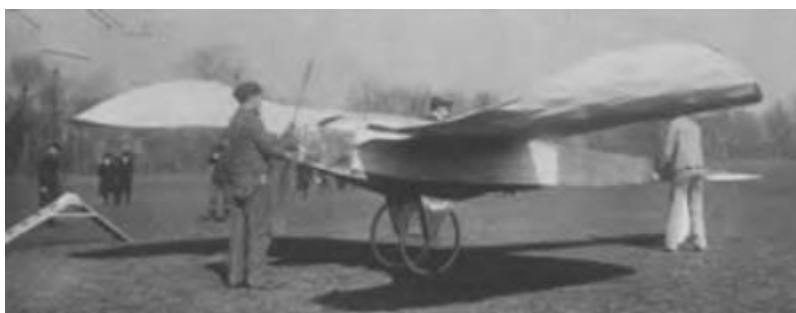
The Blériot Canard of 1907 at Bagatelle. The pilot seems to be testing the wing warping: left wing is down and the right wing up
