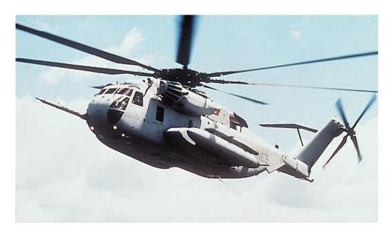
The three-engined CH-53E is the most powerful helicopter in the U.S. military inventory. The SUPER STALLION™ helicopter is cleared to 73,500 lb. with external loads. It's the only helicopter that can lift the 155mm howitzer, its crew and ammunition. It can lift aircraft as heavy as itself.
