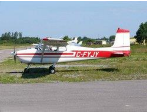
The 1957 model Cessna 172 Skyhawk had no rear window and featured a "square" fin design
