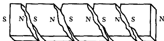
FIGURE 8-89. Magnetic poles in a broken magnet.
