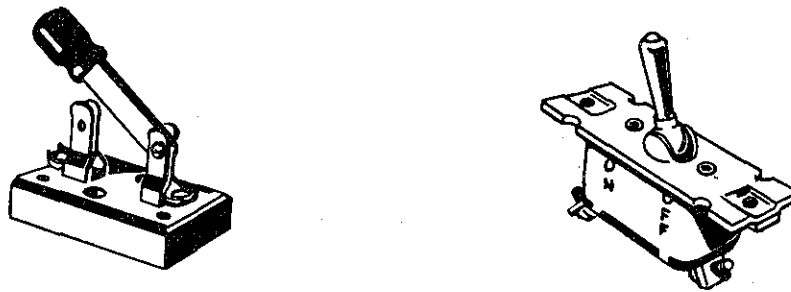
FIGURE 8-112. Single-pole single-throw knife and toggle switches.
