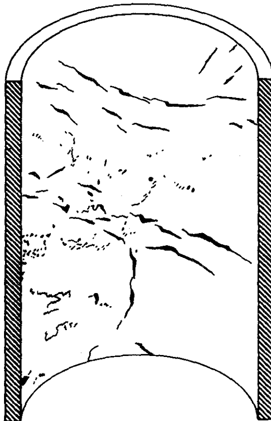
FIGURE 10-9. Heat-treat cracks on cylinder barrel wall.
