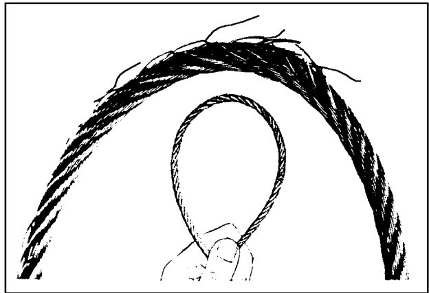
FIGURE 7-16. Cable inspection technique.
