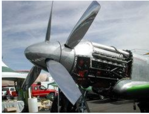
Contra-rotating propellers on a Rolls-Royce Griffon powered P-51 Mustang.
