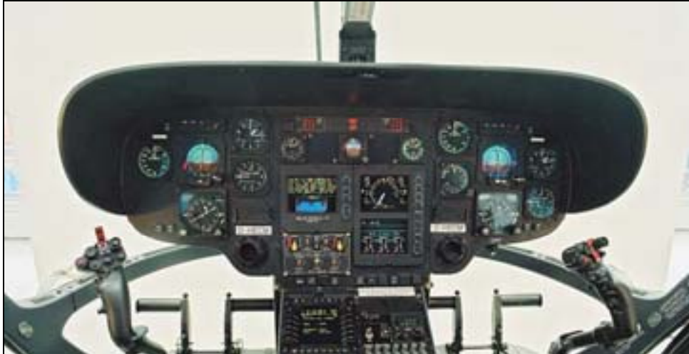
Typical example for a conventional cockpit layout (NVG friendly) .
