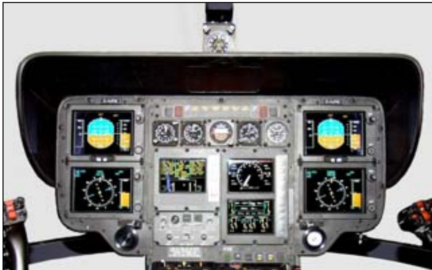
Typical example of a glass cockpit layout (NVG friendly)
