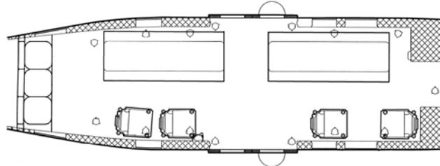
*Typical cabin arrangement, with 4 single comfort seats installed on the RH side*
