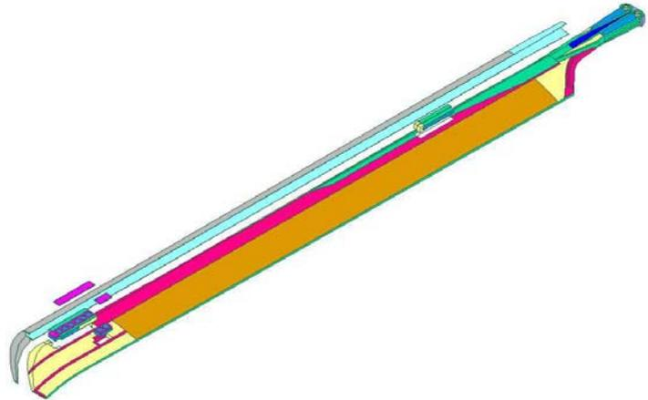
**New blade profile, multibox structure, capable of flight in icing condition**
