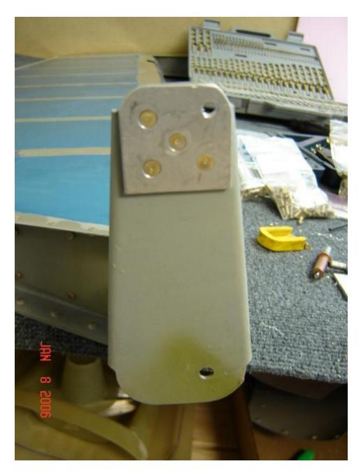
While the elevators are off the ship, I'm also going to go ahead and trim the elevator skins back to the rib in the lower area near the rudder horn. There is some potential interference with the emp deck, so I'm going to max the clearance there.
