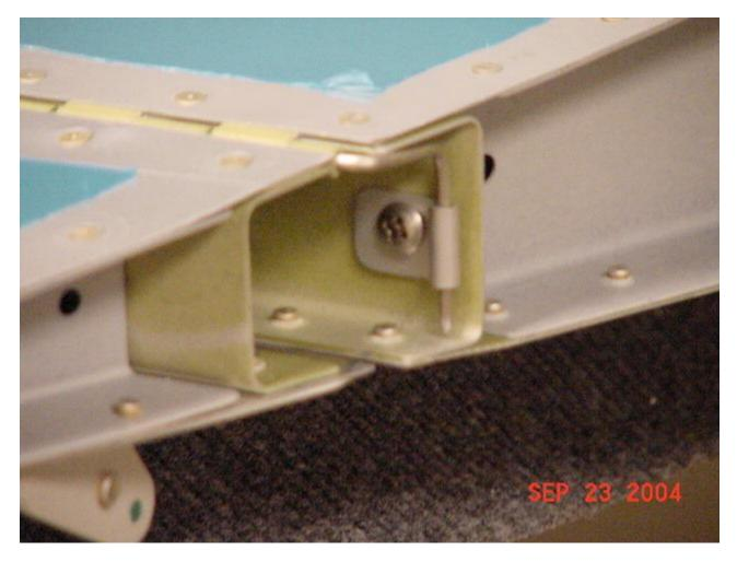
Rolling the forward side of the left elevator was pretty simple. The pre-punched rivet holes are exactly the same right and left, so I was able to use the same, now pre-drilled, piece of copper pipe. I clekoed it in, then rolled one of the three segments at a time. I started on the straight side, not the bent side. That made the job easier.
