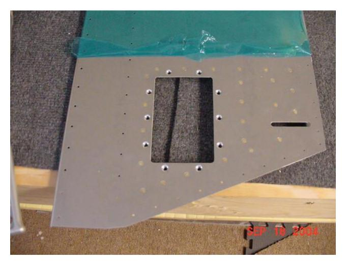
I took the Left elevator spar with the weldment clekoed to it and set it in the skins. I had already set up the counterbalance and the c/b skin, as well as the hand made bracket to hold it to the spar. I already primed the bracket, too.
