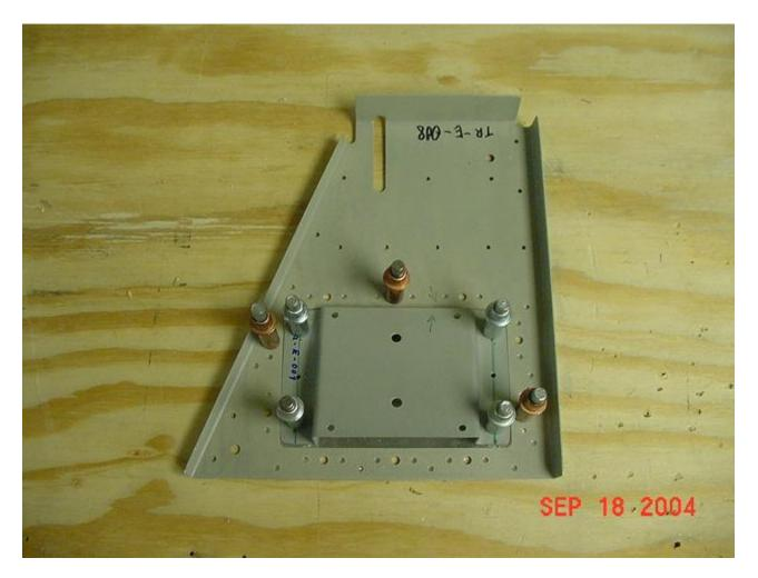
I drilled all of the attach holes on the doubler through the skin. Then I took everything apart and deburred it. I dimpled all the holes in the skin and I tried to dimple the doubler. I ended up countersinking a wee bit in the dimples on the doubler to get the rivets to sit flush. And of course for the nutplates you have to machine countersink the rivet holes.
