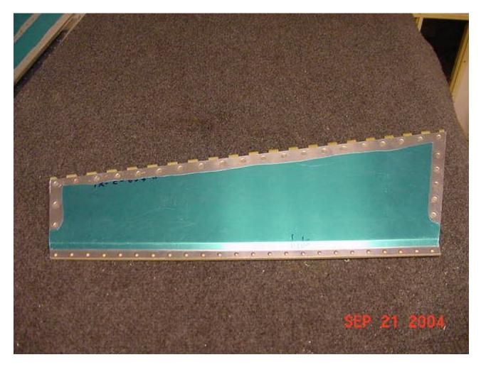
The left elevator main body is riveted like the other control surfaces. There is an area of rivets that is not accessible after you close the skins over the skeleton. Therefore you have to rivet a partial row of rivets on each skin to the counterbalance skin.
