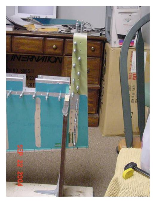
This time when riveting the counterbalance skin to the elevator skin, I used a hand squeezer instead of back riveting. I clekoed EVERY hole common to all three parts and flipped the assy with the stiffeners face down just off the edge of my table. I removed each pair of clekos and squeezed the one rivet in the bottom row (the top row goes into the skeleton.
