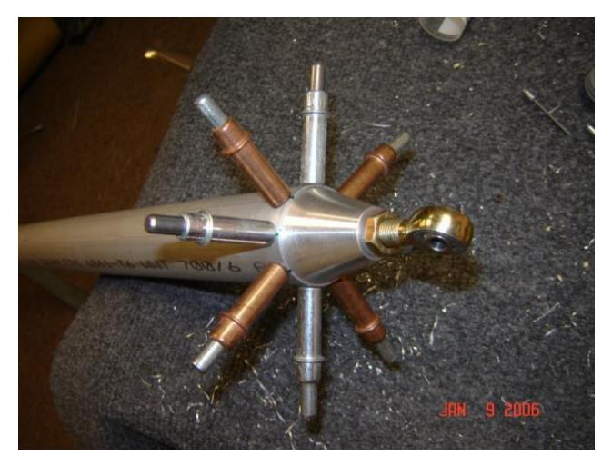
That was a fun little project. I put the aft tube in the emp, released the clamps on the elevators and checked the travel. I get about 28 degrees down, so I'm good to go there. I only get 17 up, though. Regrettably, that's because I forgot to cut the emp deck panel right after I put the angle bracket back there to hold the VF. But the bell crank does NOT hit the bulkhead so that tells me I'm really in pretty good shape with the control system. Waiting for the part, and on to other things....
