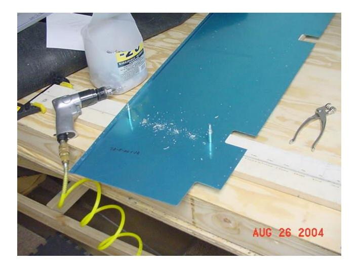
You can't see it in this pick, but the angle/stiffener is under the skin between the two boards. You spot the red mark on the green line and drill, then cleko, the first hole. Then rotate the skin until you see the green line in all the other stiffener holes and drill the trailing edge end. On the shorter stiffeners I didn't bother to cleko any other holes, just each end, prior to drilling.
