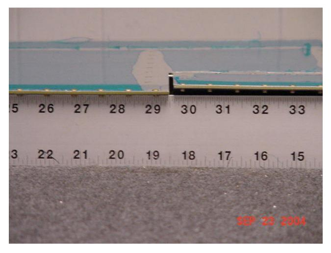
After completion of the riveting on the elevator, I couldn't wait to trial fit the trim tab. I tried to slide the pin in and it wouldn't go all the way through. Manhandling with my palms was useless. I put the hinge down against the table top and "coaxed" it a little to line the hoops up better. That got the pin all the way in fairly smoothly. Then I found out that the trailing edges did not line up very well.
