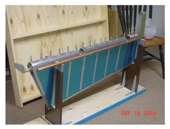
I ended up drilling and clekoing every hole. I used two pairs of Visegrips to grab the pipe in the area where the rod ends are screwed into the spar. The rod ends get in the way, so I removed them. I started at the outer edge and only clekoed one of the three segments at a time. That makes it much easier to roll.
