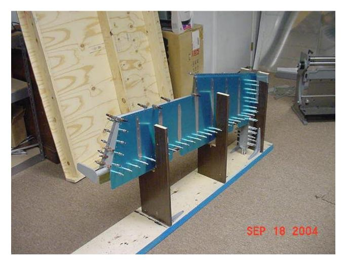
I took the E-006 spar out of the assy and took it to the bench. I got out the appropriate hinge material and rough fit it to the spar and the corresponding area on the elevator.
