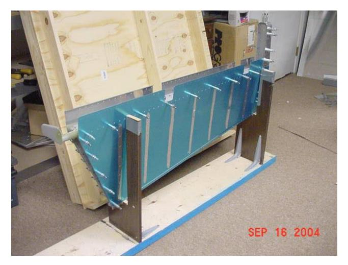
I unclekoed the R elevator and removed all of the parts from the fixture. I D&D'd the bare parts, scotchbrited them and used a self etching primer on them. I filed the edges of the skins.
