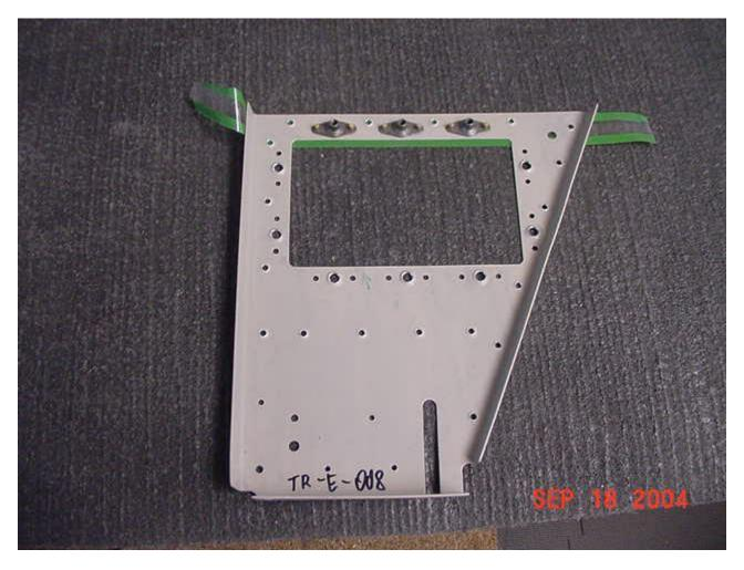
I went ahead and used my Main Squeeze and set the #3 flush rivets to hold down the nutplates. I went ahead and primed the skin where the doubler will attach. Then I clekoed the trim servo doubler to the skin. I hand squeezed all of the attach rivets for the doubler.
