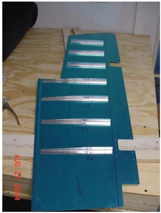
\*\*\*Note: The plans do not say, but Mark F. confirmed that the taper on the stiffeners is to 1/8" at the doubler/trailing edge end, and is cut back 6 inches toward the spar.
