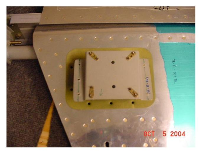
I finally got back to working on the trim tab. I didn't have the correct nutplates, so I made an order for #6 screw "end" nutplates. Once they were in hand, I grabbed the trim tab bracket and riveted the nutplates with #3-3.5 flush rivets. I screwed down the servo and riveted the bracket to the cover plate with #3-3.5 flush rivets. This was kinda fun!
