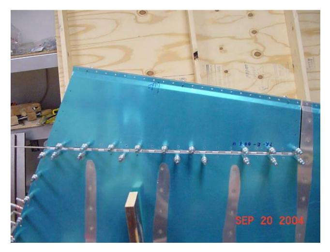
The trim tab is actuated by a rod from the servo on the bottom of the elevator. You have to put a bracket consisting of two pieces riveted together and riveted onto the trim tab. Both pieces are supplied and cut very close to shape. I used one existing skin hole and one new hole for the small piece. For the larger actuator bracket I had to drill all new holes that also go through the root rib. You also put one rivet in where the tabs of both brackets mate together.
