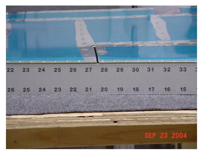
As I suspected, even riveting the "in betweens" wanted to cause the bow to return. I did a few things to fight this. I ran a drill bit through the holes biasing the direction I wanted to put pressure. I also tried to hold the trim tab with the twist I wanted (untwist, if you will...). And when I squeezed the rivets, I tried to press them the direction I need to bend or correct the trailing edge. It worked. With a little more coaxing, of course. Matt Happy!
