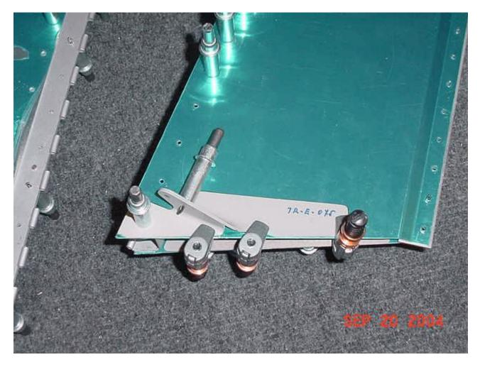
The Trim tab was fun to assemble. After D&D'ing the entire left elevator parts pile, I clekoed the trim tab components and set various sizes of #3 flush rivets, and one #4 rivet in the actuator arm brace. I set all these rivets by hand with my new Main Squeeze. So far, that thing works VERY nicely. And is more kind to my delicate hands/fingers. And the quick change feature using pneumatic type yokes is great. Anyone want to buy my Tatco squeezer?
