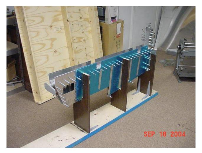
Finally the perimeter of the left elevator was all drilled @ 40 and clekoed. At this point I did things a little differently.
