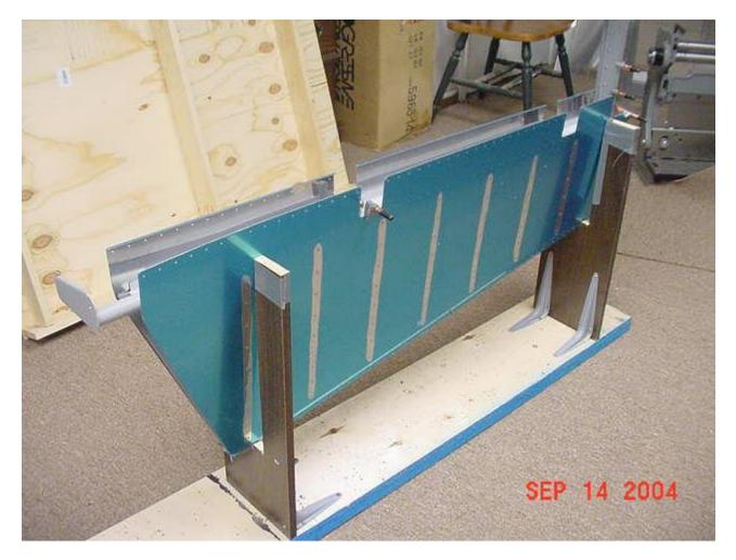
I put the trial fit R elevator assembly on the bench and measured the counterbalance skins for rivet drilling. I made sure all the flange centerlines were visible through the pre-punched holes and made sure all the parts were properly aligned per plans. I then drilled using a #40 bit, clekoing as I went along.
