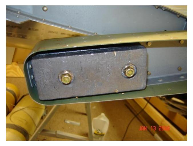
In final assembly, I will get at least one thread showing on the nuts per aviation practices. At this point I am considering leaving all 5 blocks in the elevators in tact. If one side ends up light, I will switch the weights side to side. If the elevator CW isn't heavy enough, then I will cut one of the weights and bolt each half to the forward bolt hole in the elevator CW. I'm not going to worry about that until after I have the parts painted and ready for final install.
