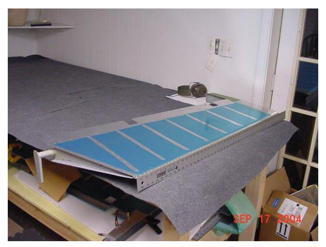
The R elevator went back in the fixture and I stared at it a bit. I have to roll the leading edge of the skins and rivet them together in a curve (where the rod ends bolt/swing on the HS). Plans say to us duct tape or cleko a 1" pipe to the skins and roll them until the pre-punched holes line up. I didn't have
