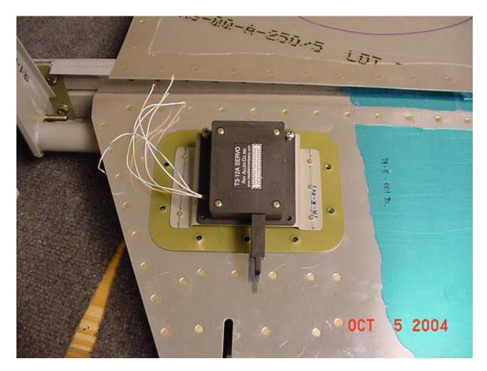
Once the servo bracket and cover were in place, I played with the activation rod a bit, just to make sure it cleared through the hole.
