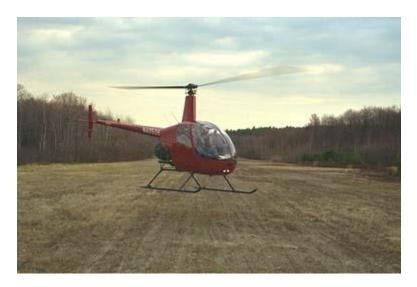
This photo shows the helicopter has descended most of the way to the ground, using the energy stored in the spinning rotor system to provide thrust. About this height is where the pilot will raise his collective pitch control all the way up in order to get every bit of available thrust to cushion the landing as much as possible.
