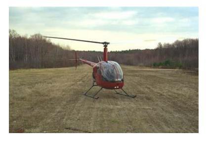
Notice the coning of the rotor blades in this final picture. They make a distinct "V" shape because there is no longer sufficient RPM to hold them down straight.
