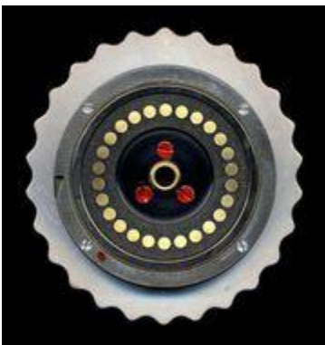
The left side of an Enigma rotor, showing the flat electrical contacts. A single turnover notch is visible on the left edge of the rotor.
