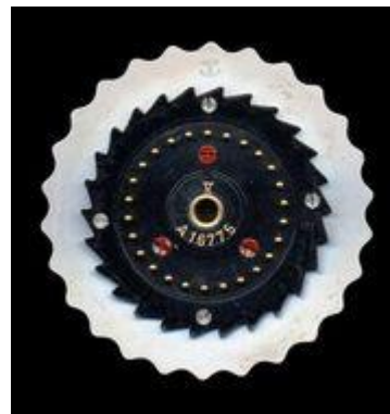
The right side of a rotor, showing the pin electrical contacts. The Roman numeral V identifies the wiring of the rotor.
