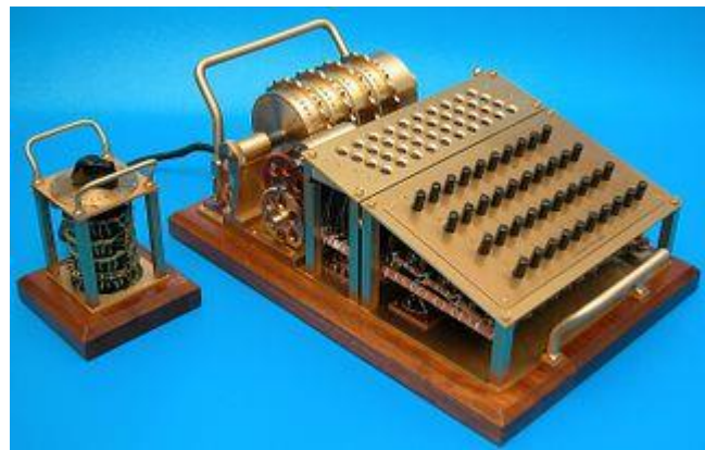
Tatjana van Vark's Enigma-inspired rotor machine, constructed in 2002. The rotors of this machine contain 40 contacts, compared to the original Enigma's 26.
