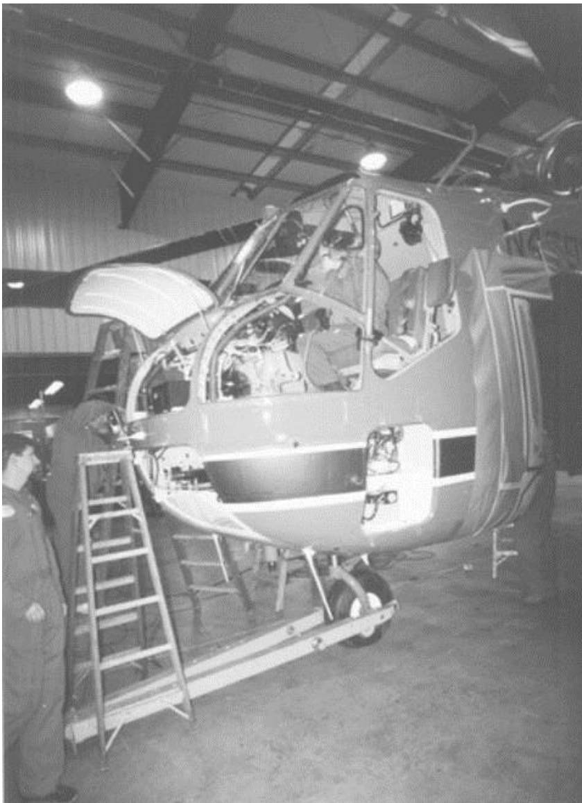
Technicians completing final avionics adjustment on the Aircrane before test flight.
