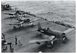
Prior to the first flight of the XF4U-1 the Navy commissioned Vought to study a night fighter, version of the F4U-1. Working with the Sperry company and the MIT Radiation Laboratory the necessary radar equipment needed to accomplish the mission was developed and the necessary Engineering design modifications determined for conversion of the F4U-1 to the F4U-2 Night Fighter.
