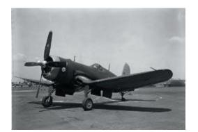
on the outer panel wing mounts. Twin pylons located on the wing center section could carry either two 150-gallon drop tanks, two 1,000-pound bombs or two big 11.75-inch rockets.
