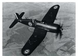
an F4U-4 in an F4U-6 (AU-1) airframe, it was equipped with a Pratt and Whitney two-speed, two-stage engine (R-2800-18W), making it a high-altitude fighter.
