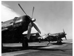
The gull wing F4U-4 was equipped with a Pratt and Whitney R-2800-18W, a 2100-horsepower engine with a two-stage supercharger and a new Hamilton Standard four-bladed, 13-foot-2 inch diameter propeller, it was rated a 446-mph fighter. It arrived on the battlefront in June of 1945 for the final push against the Japanese mainland.
