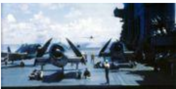
Grumman F6F-3 Hellcats on the flight deck with wings folded, Grumman Avenger on landing approach
