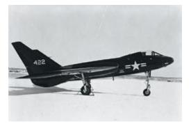
The carrier suitability testing, which was completed in August 1951, essentially doomed further production of the F7U-1 and led to the design of a completely modified F7U, the F7U-3. F7U-1's were used extensively for flight-testing and were flown briefly by the Navy Blue Angels Demonstration Team.
