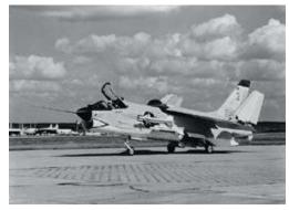
Control and guidance equipment for the Bullpups was mounted on the upper surface of the wing center section and enclosed in a "humpback" fairing.
