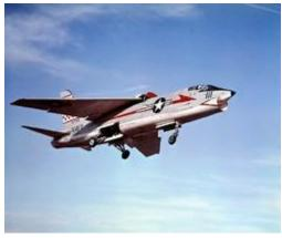
version. This version of the Crusader was identifiable externally by the new radome configuration - an all plastic radome in lieu of the combination metal/plastic radome of the F8U-1. The new radome had a small glass window on the lower aft surface which permitted a gun camera to record the results
