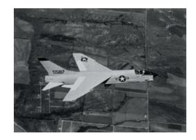
The higher-thrust-rated engine P-16 engine resulted in an increase in the maximum speed of the aircraft to 960 knots. This, combined with a nagging yaw problem at high altitude experienced on the
