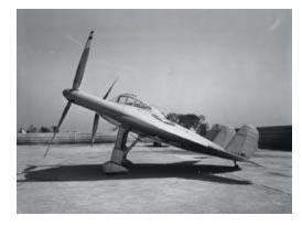
The pilot could enter or egress from the cockpit through a hatch in the cockpit floor or through a sliding canopy.
