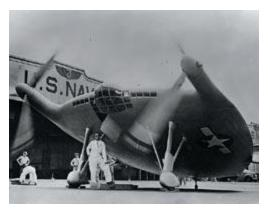
For light weight, the airframe structure was made of wood with fabric covering. With a wing loading of only 5 lbs/sq ft, the V-173 could lift off in 200 feet in a calm, and with a zero run against a 25-knot headwind. However, with a power loading of 14-lbs/hp maximum, level flight speed was only 138 mph.
