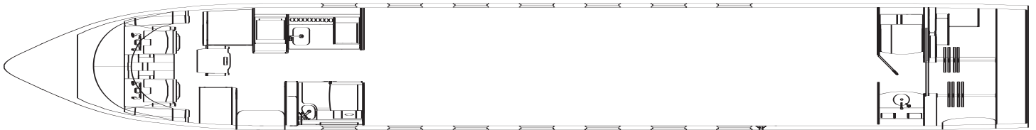
The Forward Galley without Crew Rest
