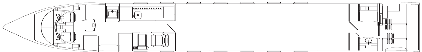
The Forward Galley with Crew Rest
