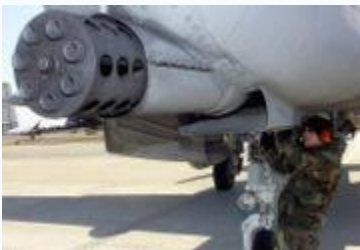
The GAU-8 Gatling gun of an A-10 Thunderbolt II at Osan Air Base , Korea.
