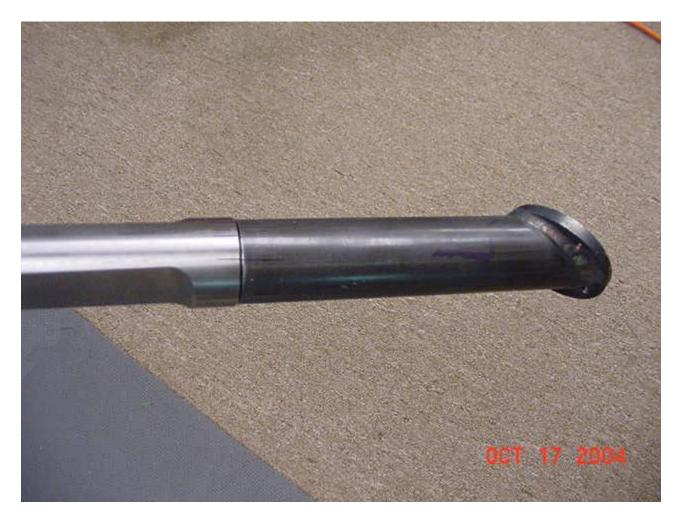
I used a ruler and marked several lines across the gear leg and foot. This gave me a way of making sure I kept the leg and foot in alignment. One foot was extremely tight and did not want to wander, but the other foot could move fairly freely. This was a potential problem during drilling.
