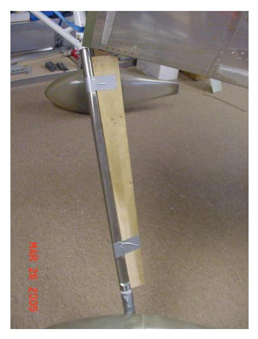
What I plan to do is just to slice a bevel on the wood near the fuselage and ProSeal (or GOOP) the wood dampers to the titanium legs.
