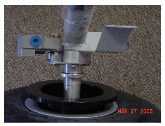
Contrary to what the TR plans recommend, I am probably making all of my hydraulic lines out of 1/4 inch Nylaflow tubing. I've had aluminum lines break 3 different times on other planes, so I'm making the switch to nylon. With brass fittings. The burst pressure is at least 1000 pounds, and I've been told that you can't put that much pressure on a brake line with your feet and legs. So I'm going plastic.
