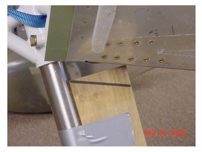
I think if you leave the corner on there, it's going to interfere in service, plus the damper will extend over the steel foot. The cut might make fiberglassing the tape over the leg a bit easier,too. I think it will work. I checked the fairings over the dampers already and it should all fit together.
