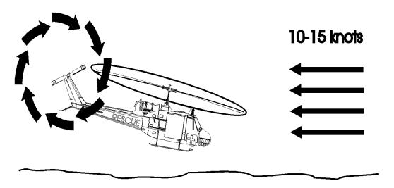
Effective Translational LiftAt airspeeds between 10 and 15 knots, depending on the model of helicopter, the rotor completely outruns the recirculation of old vortices and begins to work on clean air. Effective translational lift results.
