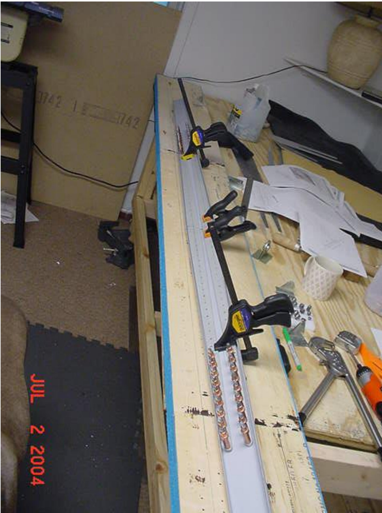
I flipped the clamped assy over on it's side, resting on the clamps, drilled 4 holes, flipped the assy back over again, clekoed everything down and finished drilling the holes.
