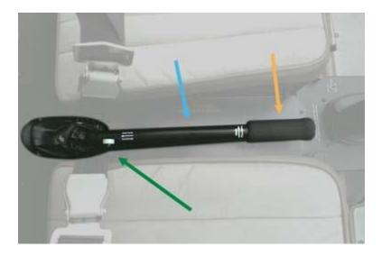
The blue arrow points to the collective lever (which the throttle twist grip is mounted on). The collective lever is connected to the swash plate by a series of push-pull tubes. Raising the collective lever increases the pitch on the main rotor blades, lowering the collective lever decreases the main rotor blade pitch.
