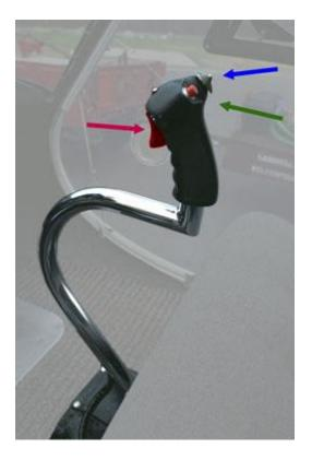
The arrows are pointing to 3 controls on the F28 cyclic.
