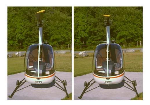
In this picture, you can clearly see that the angle of the blade with respect to the horizon has changed, from a nose up angle on the left side, to a nose down angle on the right side. In this case, the swashplate has moved in response to either the cyclic, collective, or both, and has moved the
