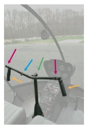
There are a few things to note, which is why there are so many arrows! The orange arrows point to the hand grips. The green arrow points to the pivot point for the cyclic. The hand grips can be teetered up and down around this pivot, like a see saw. If one hand grip goes up, the other has to go down, they can't move independently.
