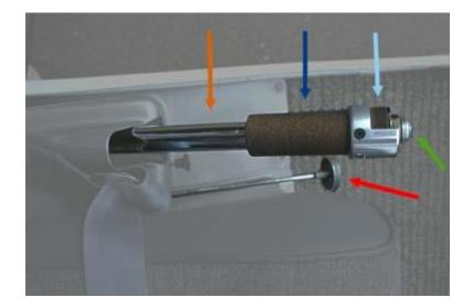
The orange arrow points to the collective lever, which works identically to the collective lever on the Robinson.
