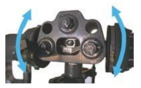
It is important to understand that teetering happens "automatically", as a result of aerodynamic and centrifugal forces. The pilot does not command flapping with the control system.
