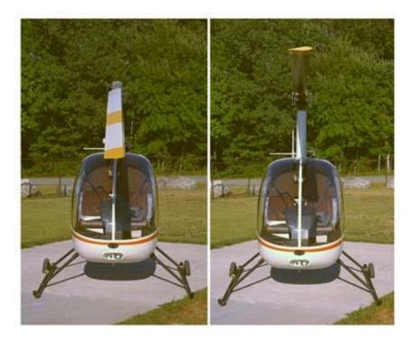
Notice that the angle the airfoil makes with the horizon here does not change. Flapping changes the angle of attack not by pitching the airfoil up or down, but by changing the direction of the wind relative to the blade. For a more in-depth discussion see <u>Relative Wind</u>, <u>Flapping</u> and <u>Angle of Attack</u>.
