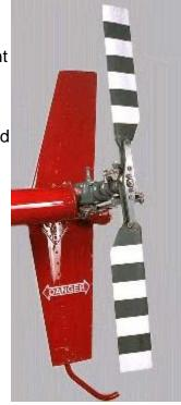
counter the rolling tendancy, the tail rotor blades are typically allowed to flap, eliminating the lift dissymetry. Here is a picture of a Bell 206 JetRanger tail rotor flapped to right and left extremes:
