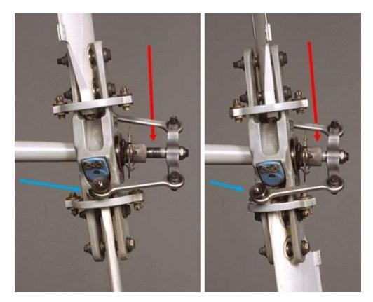
As the inner shaft slides left and right, the pitch change rods are dragged along, and pulls the blade pitch change horn along with it. The blue arrow points out how far the rod end has moved, taking the blade's leading edge with it. Like the Robinson, the blade is mounted on two spherical bearings, which cause it to rotate only in the pitch axis.
