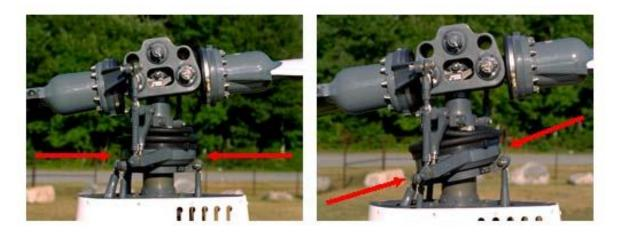
Notice that the swashplate in the left hand photograph is basically level, while in the right hand photograph it has been tilted. The tilt will cause the pitch link to have to move up as it travels to the right hand side of the picture, and move back down as it travels to the left hand side of the picture. As it moves up and down the blade pitch will increase and decrease.
