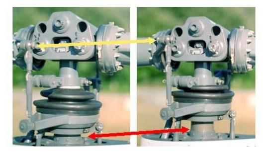
You can see that the red arrow is pointing to the bottom of the swashplate in the left hand picture, but that in the right hand picture the entire swashplate has moved up the mast. Notice the effect that has
