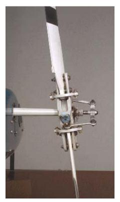
Here is a closeup of the tail rotor hub at two extreme pitch settings. In the left hand picture, the red arrow shows that the inner shaft has been extended all the way to the right. The right hand picture shows the same shaft has been retracted:
