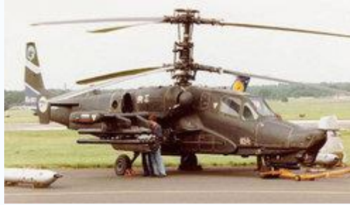
Kamov Ka-50 helicopter with contra-rotating co-axial rotors.
