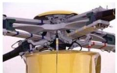
After the torque effect, the other main problem was the **tendency of the helicopter to roll laterally in the direction of the retreating rotor blades** as the advancing blades pass through denser air and generated greater lift than the retreating blades that pass through less dense air.
