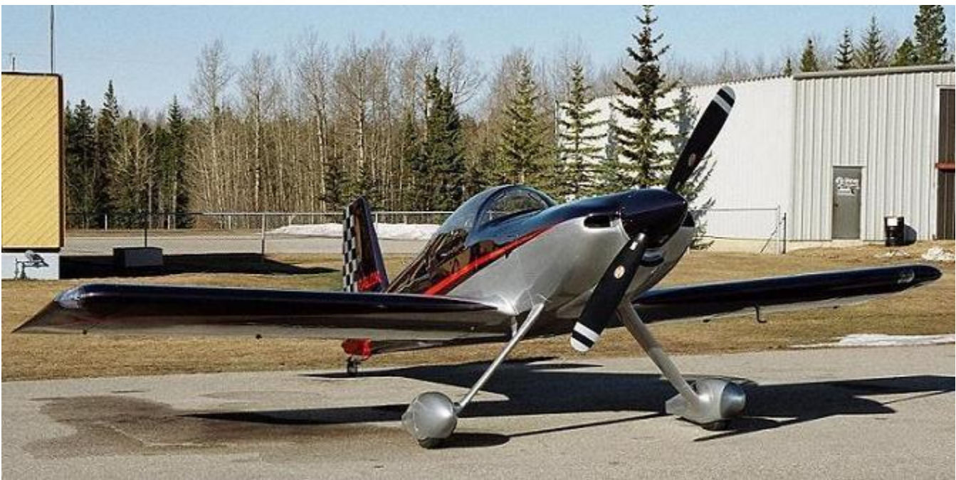
Yet another new F1 Rocket from Canada, below is Mark Esterhuizen's kit #85, complete with TACS (Taxi Aid Camera System). Yes, the nose is a little high on these birds, and unless you have a forward looking camera (or periscope) on the ground, S turns while taxiing are mandatory.
