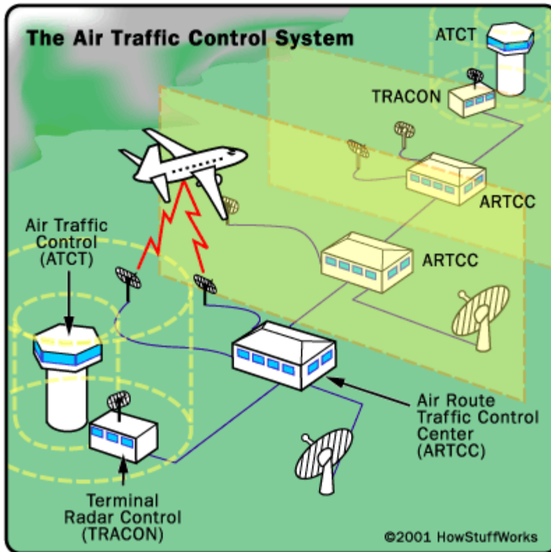
The various air traffic control facilities encountered by a plane during its flight
