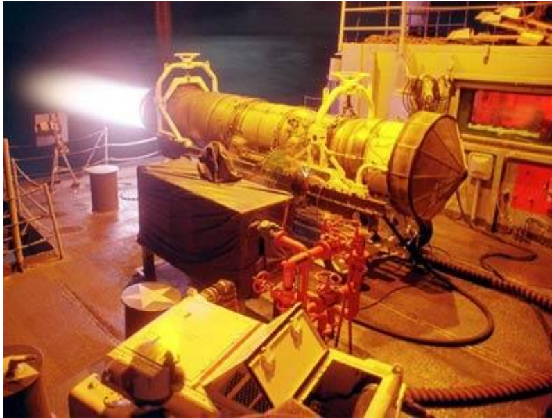
Photo courtesy U.S. Navy Testing an F-14 engine on the fantail of the USS Kitty Hawk
