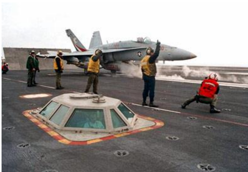
Photo courtesy U.S Department of Defense Steam rises from the catapult as an F/A-18C Hornet prepares to launch from the USS George
