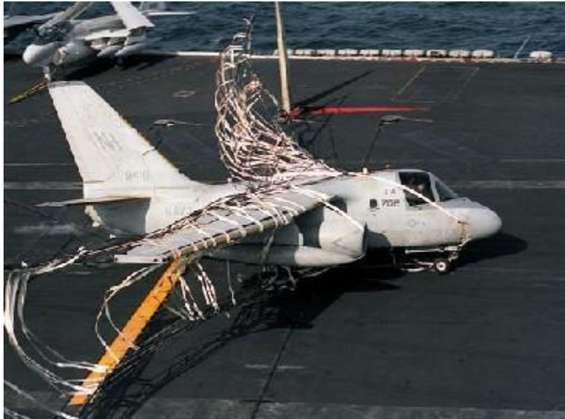
Photo courtesy U.S Department of Defense An S-3A Viking aircraft lands on the USS Abraham Lincoln with the help of the crash barricade. The plane had to make an unconventional landing due to a problem with its landing gear.
