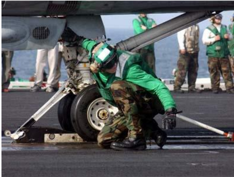
Photo courtesy U.S Navy A member of the USS George Washington flight-deck crew checks an F-14 catapult attachments. Tomcat.
