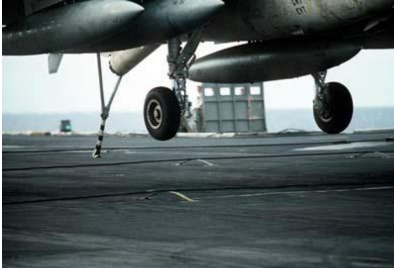
Photo courtesy U.S Department of Defense The tailhook of a KA-6D Intruder aircraft, about to catch an arresting wire on the USS Dwight D. Eisenhower
