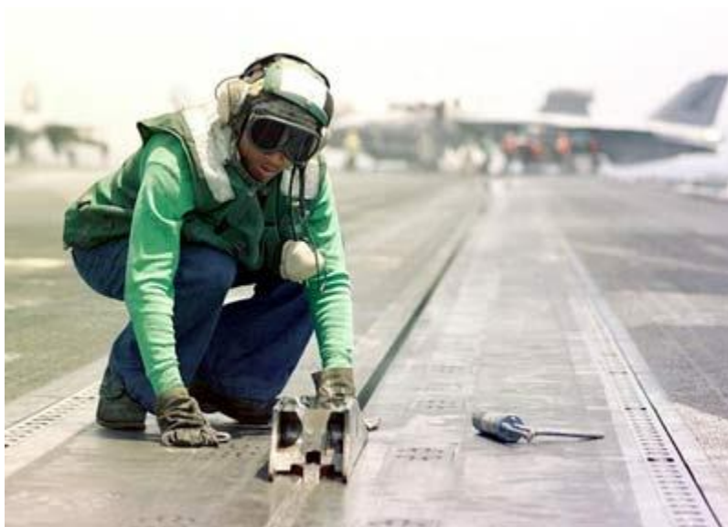
Photo courtesy U.S Department of Defense The shuttle of catapult number four on USS John Stennis
