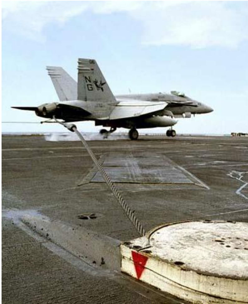
Photo courtesy U.S Department of Defense An F/A-18C Hornet catches an arresting wire on the USS Nimitz.
