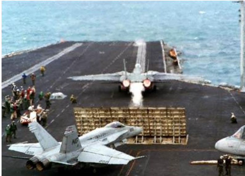
Photo courtesy U.S Department of Defense A F-14 Tomcat, positioned in front of the jet blast deflector on USS Nimitz's catapult #1
