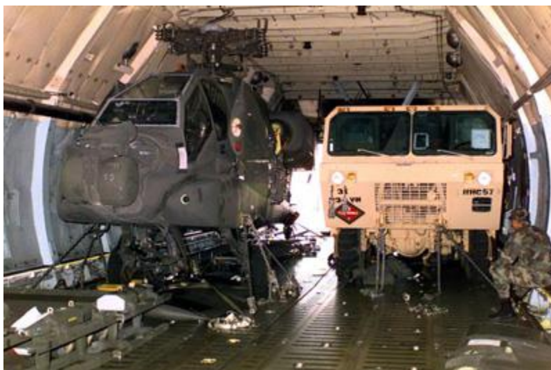
Photo courtesy U.S. Department of Defense The Apache's blades and wings detach for easier transport.
