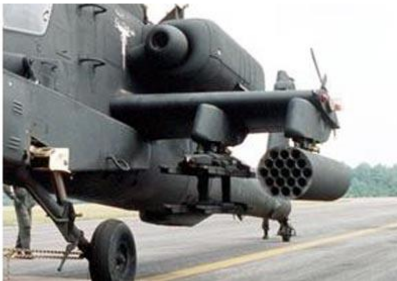
Photo courtesy U.S. Department of Defense The Hydra rocket launcher (right) and Hellfire missile rails (left) on an AH-64A Apache helicopter
