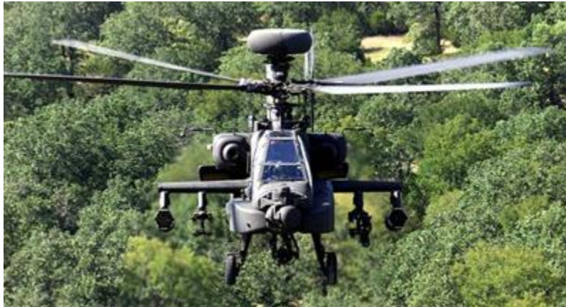
Photo courtesy U.S. Department of Defense The Apache Longbow has a distinctive radar dome mounted to its mast.
