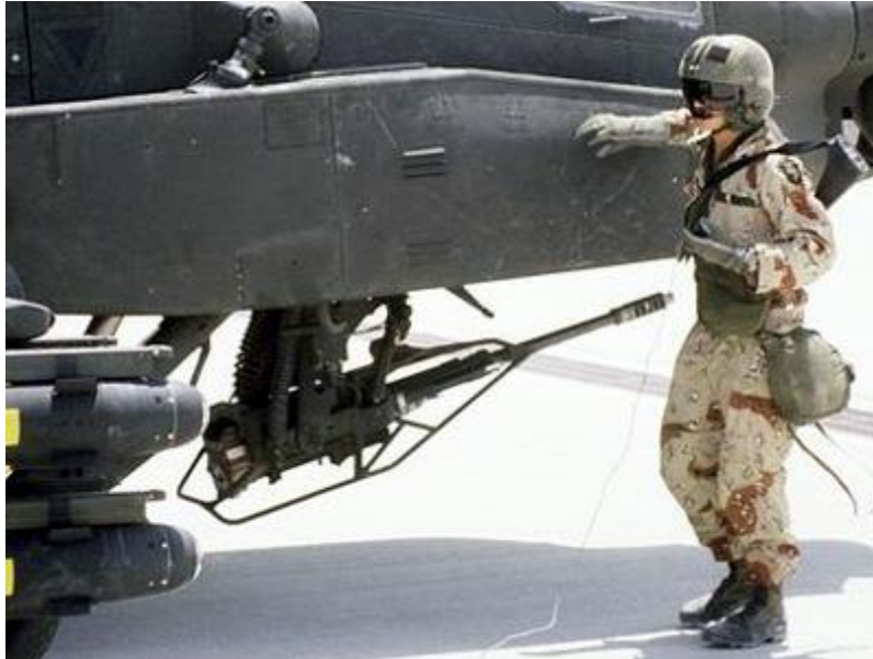
Photo courtesy U.S. Department of Defense The M-230A1 30-mm automatic cannon on an AH-64A Apache
