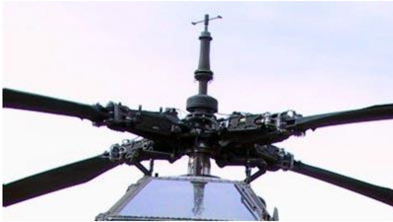
Photo courtesy U.S. Department of Defense The rotor assembly on an AH-64A Apache
