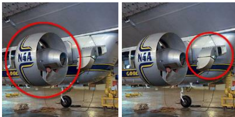
Photo courtesy Goodyear Tire & Rubber Company The engines (left) and air scoops (right)
