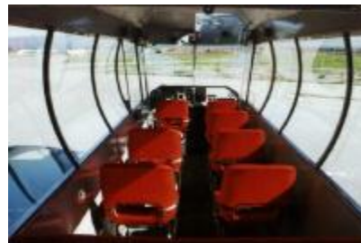
Photo courtesy American Blimp Co. Forward view inside of gondola, showing pilot seats/controls (front) and passenger seats
