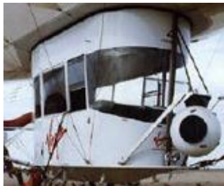
Photo courtesy American Blimp Co. Blimp gondola with an attached camera (round object in front)
