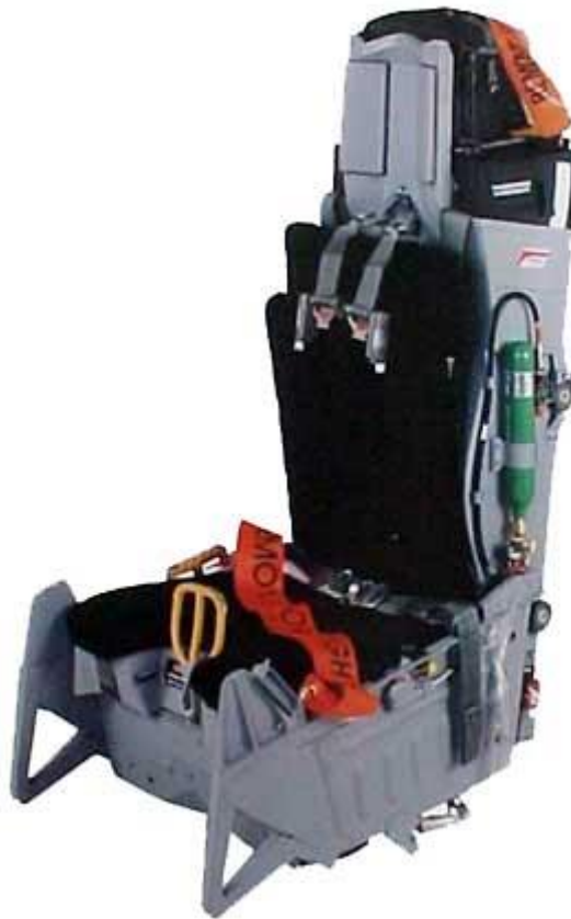
Photo courtesy Goodrich Corporation This ACES II ejection seat has a middle pull handle used to activate the ejection sequence.
