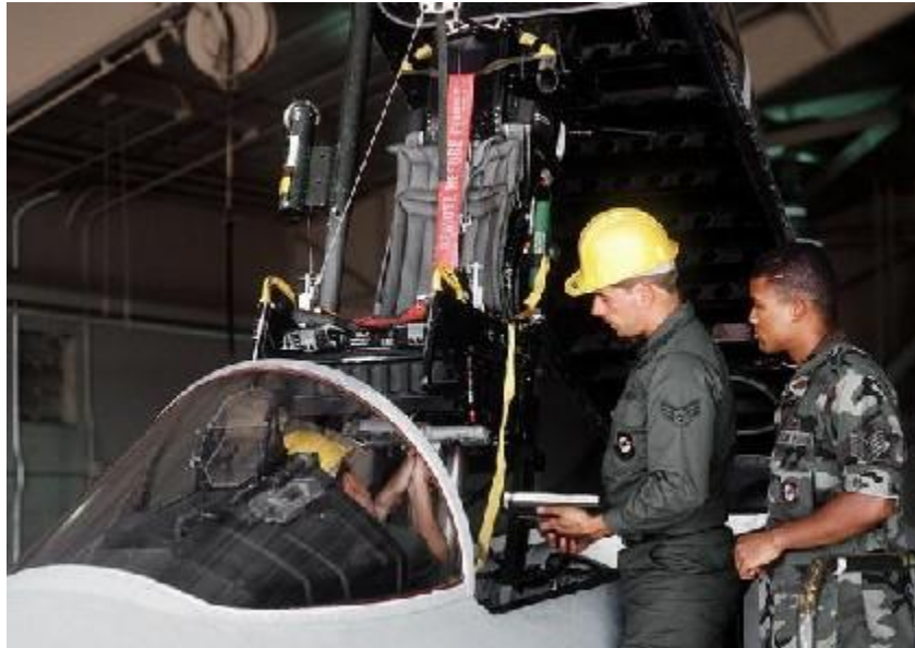
Photo courtesy U.S. Department of Defense An ejection seat being removed from an F-15C Eagle
