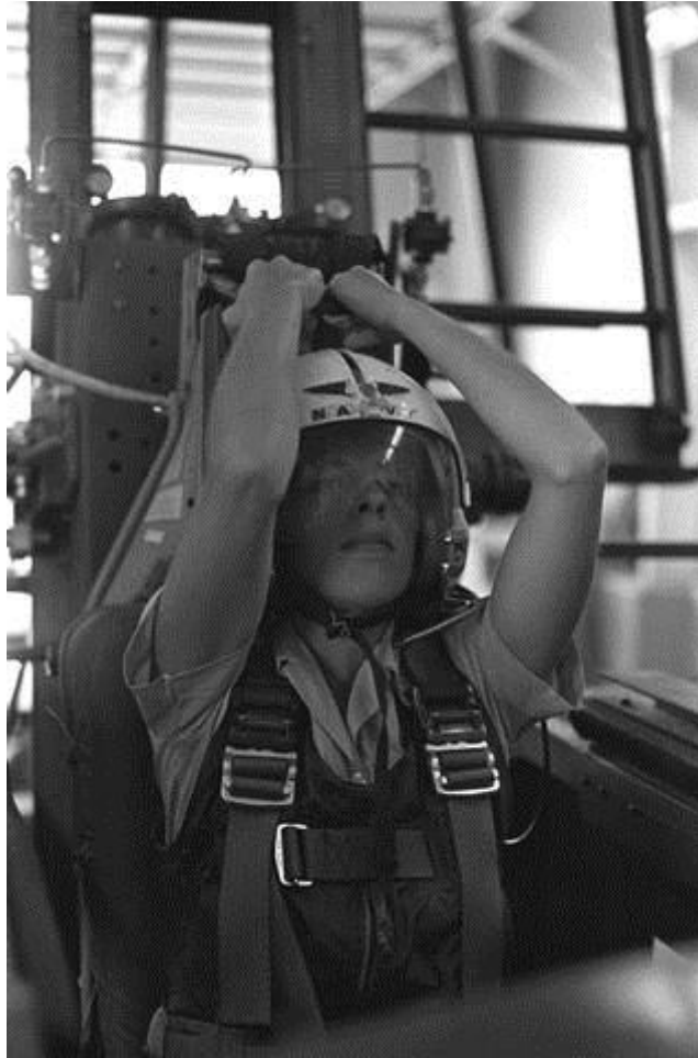
Photo courtesy U.S. Department of Defense A pilot prepares to pull down the face curtain that will launch the ejection seat up the track of the ejection-seat trainer.
