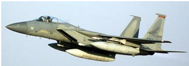
Photo courtesy U.S. Air Force The F-15 can carry extra fuel in three external tanks. One mounts under each wing and one attaches to the fuselage.
