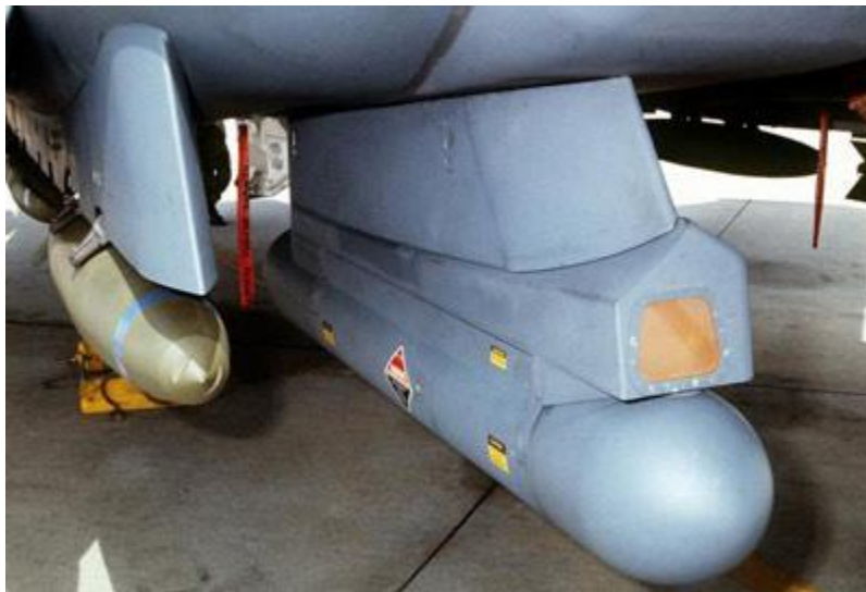
Photo courtesy U.S. Department of Defense One of the LANTIRN pods on an F-15 Strike Eagle
