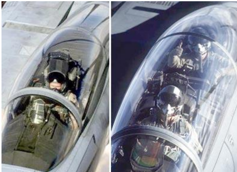
Photo courtesy U.S. Department of Defense The cockpit in the F-15 Strike Eagle (on the right) has an extra station for the weapons systems officer.
