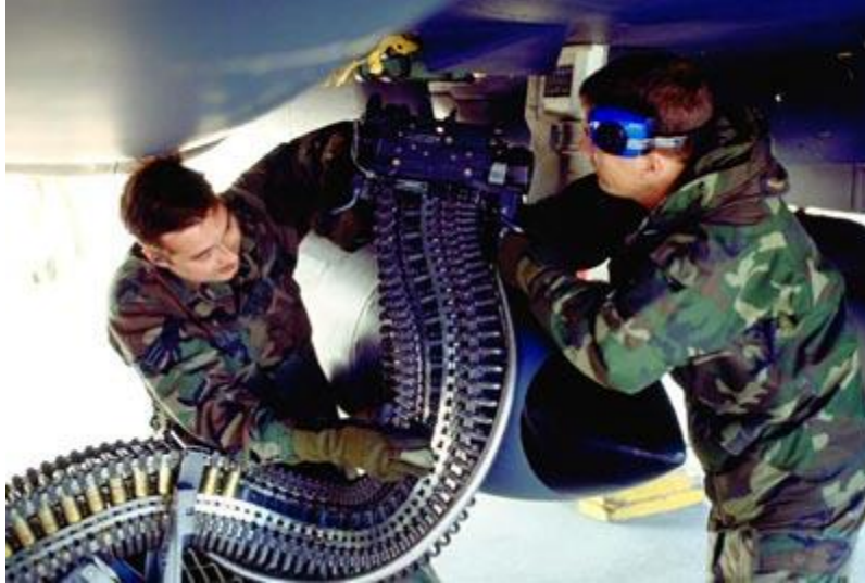
Photo courtesy U.S. Department of Defense Airmen load ammunition for the F-15's 20-mm cannon.
