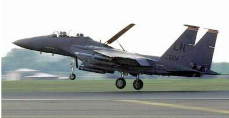
Photo courtesy U.S. Department of Defense An F-15 extends its air brake before landing.
