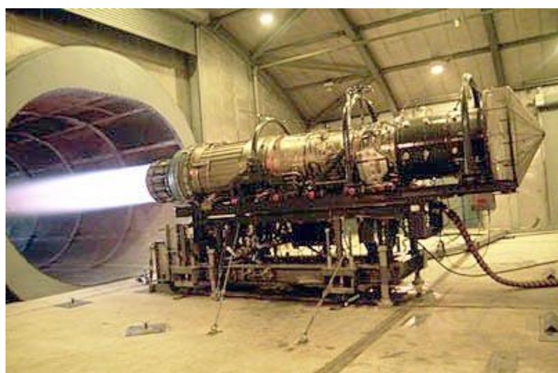
Photo courtesy Department of Defense An Air Force maintenance squadron tests out a Pratt Whitney F100-PW-220e engine configured for the F-15.
