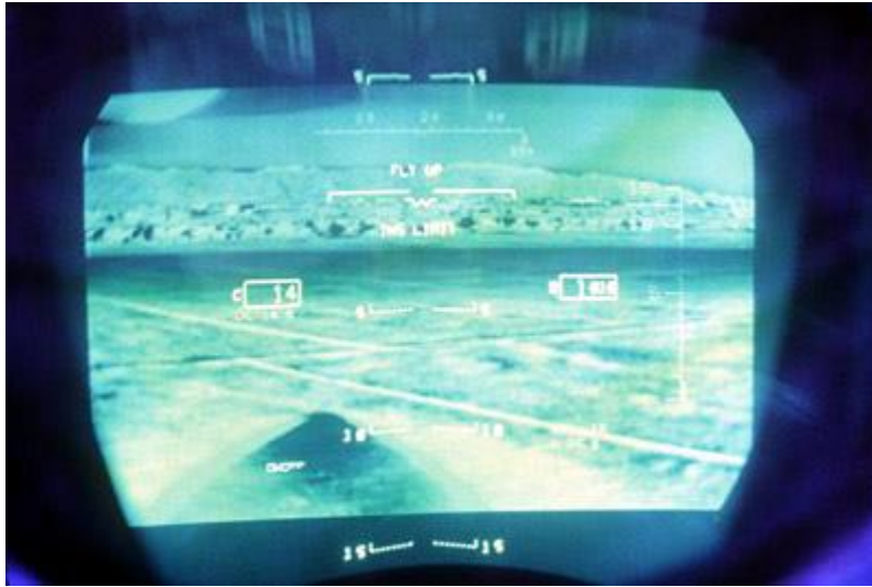
Photo courtesy U.S. Department of Defense An infrared terrain image displayed on an F-15's heads-up display
