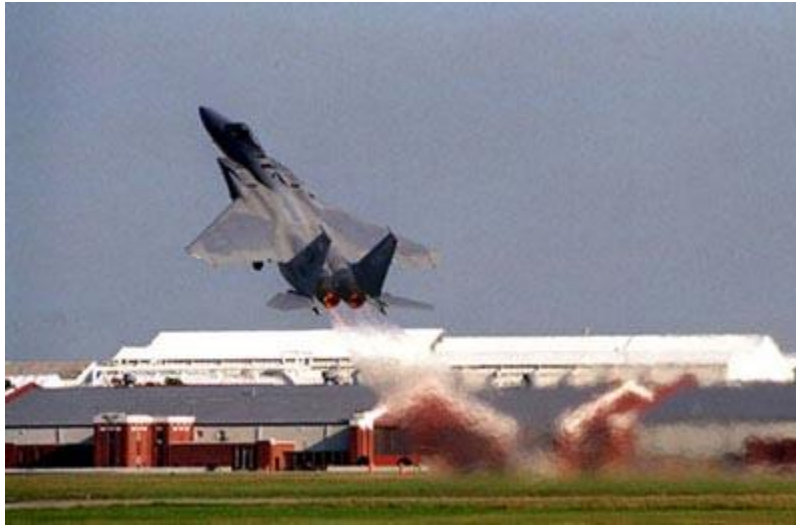
Photo courtesy U.S. Air Force An F-15's high thrust-to-weight ratio and low wing loading let it shoot off the ground at a sharp angle.
