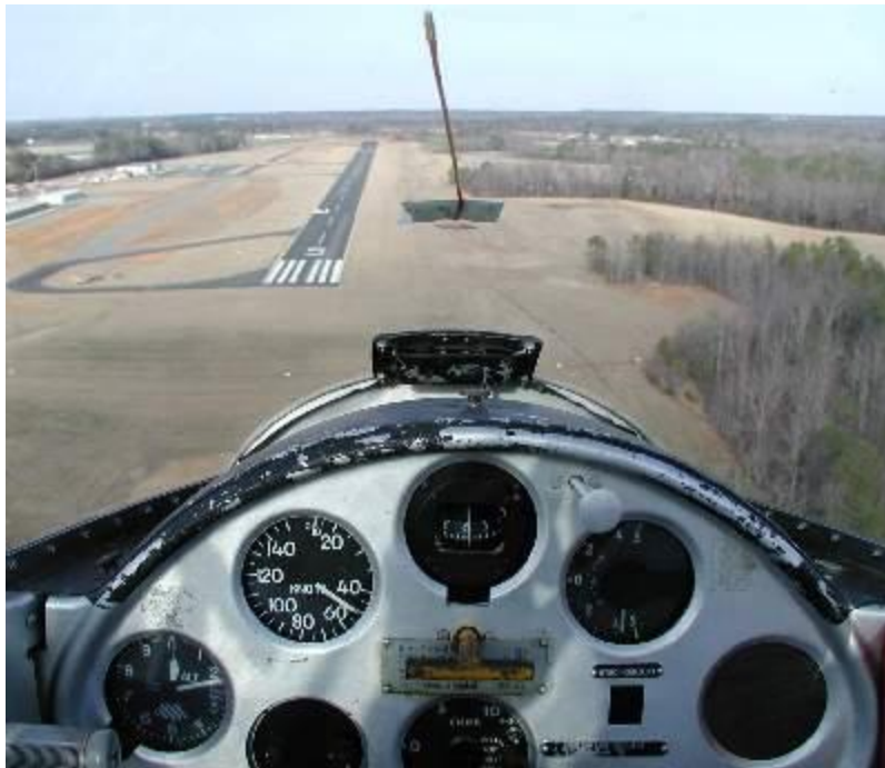
The string on the windshield tells the pilot if the plane is yawing
