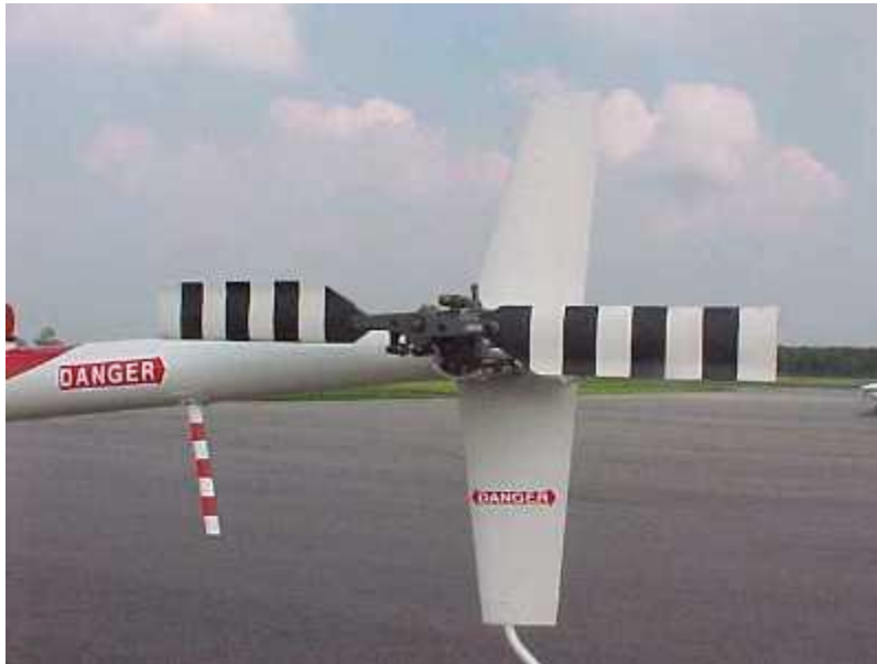
The blades of the tail rotor are only about 2 feet (61 cm) long.
