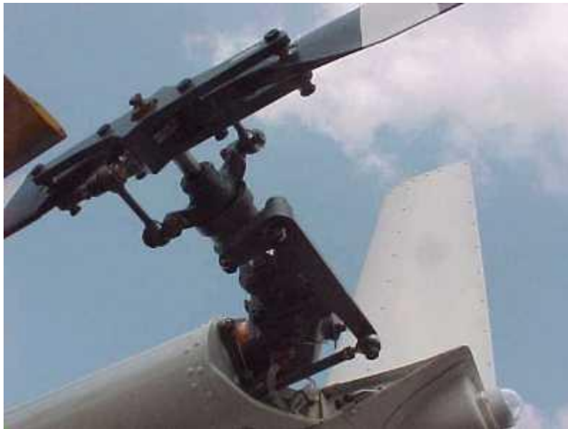
The tail rotor's hub allows the pilot to change the angle of attack of the rotor's wings.
