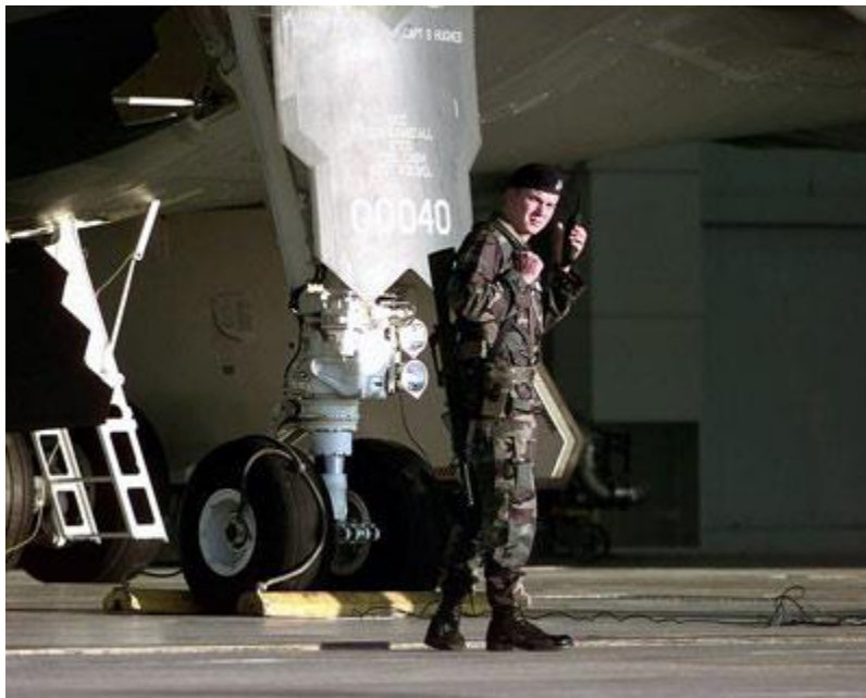
Photo courtesy U.S. Department of Defense A B-2's landing gear
