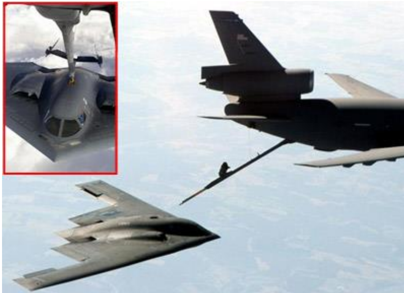
Photo courtesy U.S. Department of Defense A U.S. Air Force KC-10A extender aircraft refuels a B-2 bomber midflight.
